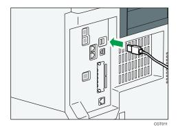
If you are using a USB interface cable, connect the other end of it to a card authentication device or media slot.
