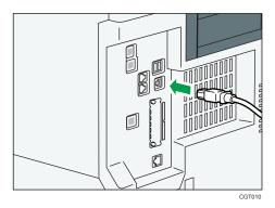
When connecting the USB interface cable to the USB2.0 (Type B) port on the Gigabit Ethernet board
