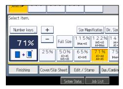
Press [—] or [+] changes the ratio in increments of 1%. Pressing and holding down [—] or [+] changes it in increments of 10%.
