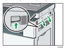
2. Push down the envelope lever of the fusing unit on the left.
