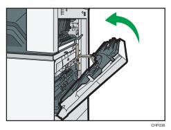
4. Open the bypass tray and set the envelopes print side down with their flaps closed and pointing toward the back of the machine. Push the envelopes into the machine until you hear the beep.
