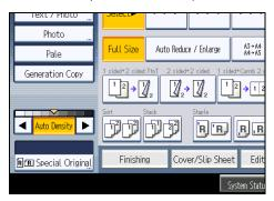
2. Press [◀] or [▶] to adjust the density. The density indicator "▽" moves.
