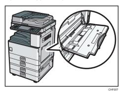
2. Insert the paper face down until you hear the beep, and then align the paper guides to the paper size.
