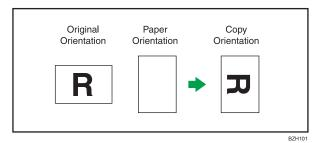
You cannot use Rotate Copy when enlarging onto A3, B4 JIS,  $11 \times 17$ , or  $8^{1}/_{2} \times 14$  size paper. In this case, place your original in the  $\square$  orientation.
