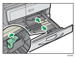
3. While pinching the release lever of the end fence, slide the end fence outward.
