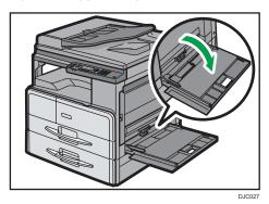
2. Load the paper face down, and then adjust the paper guide with the paper size.
