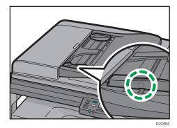
1. Place the aligned originals face up in the ADF. The last page should be on the bottom.
