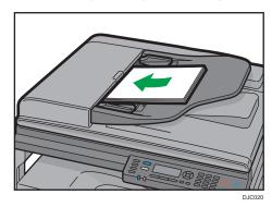
2. Adjust the guides according to the size of the original.
