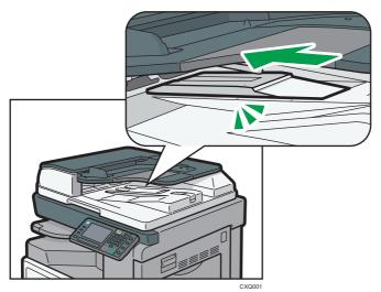
When the slide tray is placed on the left side, the tray capacity is decreased. After scanning the originals, return the slide tray to the original position.
