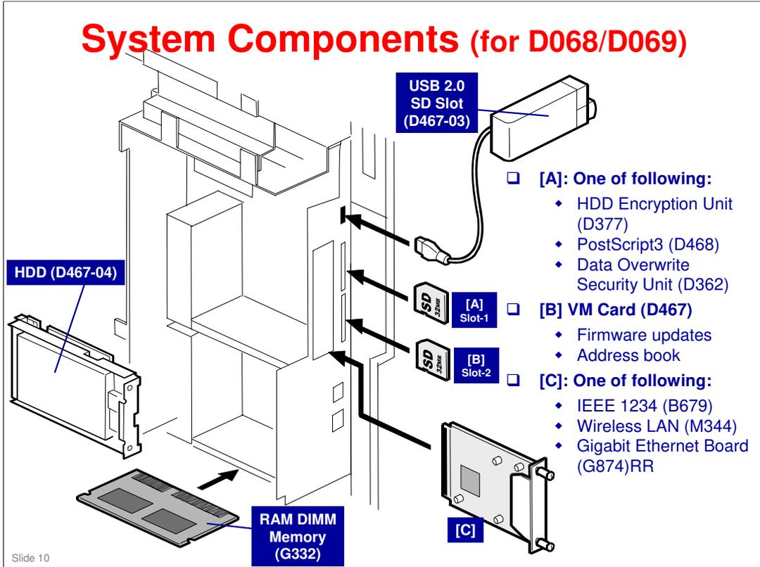
RAM DIMM memory distributed with the printer.
