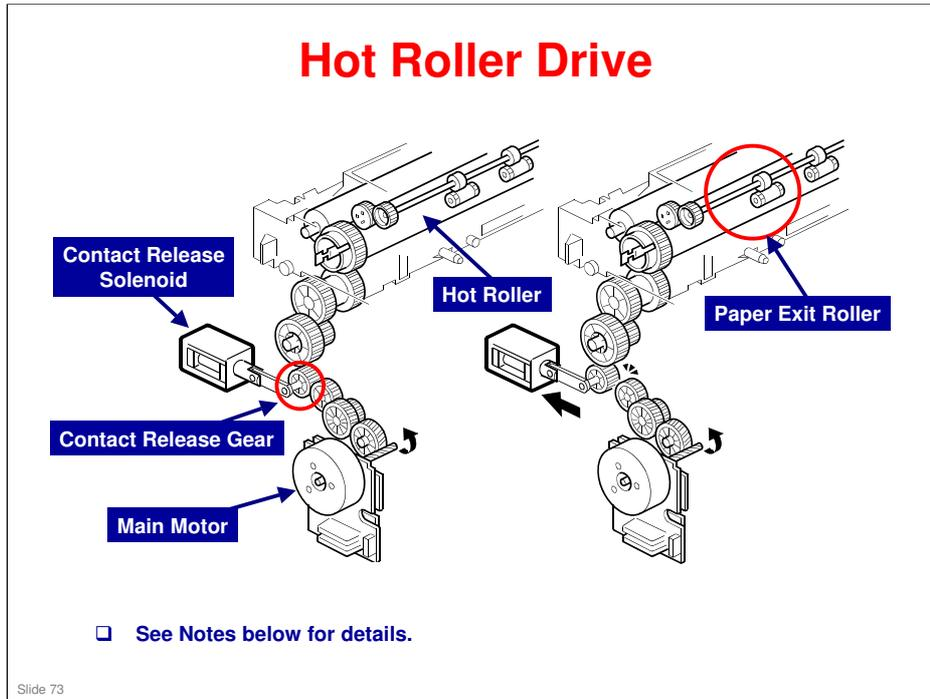
**Hot Roller Drive Mechanism**
