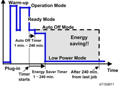
The area shaded grey in this diagram represents the amount of energy that is saved when the timers are at the default settings. If the timers are changed, then the energy saved will be different. For example, if the timers are all set to 240 min., the grey area will disappear, and no energy is saved before 240 min. expires.
