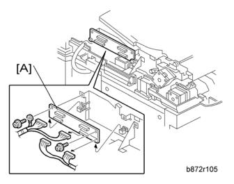
2. DF drive board [A] ( 🌶 x 2, 🗂 x 4, ground cable x 1)
