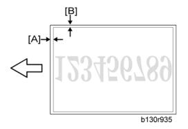
3. Measure the distance between the leading edge of the image area and the leading edge of the paper [A].
