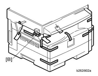
3. Remove the spacing wedge [B].
