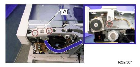
3. Remove the right platen stay holder [A] (  ${\ensuremath{ \ensuremath{\mathcal{P}}}} x$  3).
