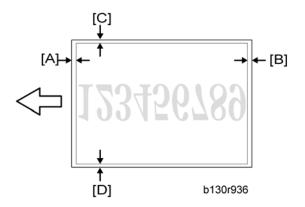
Measure the distance between the four edges of the image area and the four edges of the paper [A] [B][C][D].
