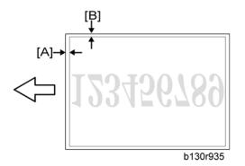
Measure the distance between the leading edge of the image area and the leading edge of the paper
