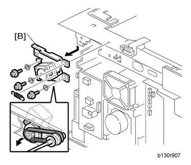
4. Scanner motor [B] ( 🌶 x 3, 1 spring, 3 screw holders, 🖽 x 1)
