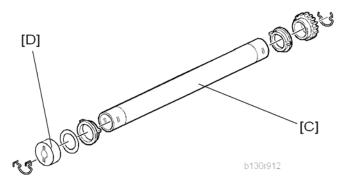
4. Hot roller [C] (2 C-rings, 1 spacer, 1 gear, 2 bushings, 1 cover [D])
