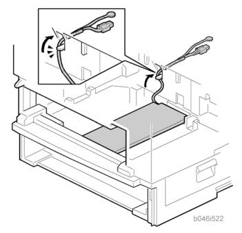
23. Pull the excess length of the heater's harness out the opening at the rear.
