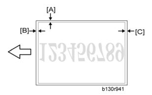
4. Measure the distance between the side edge of the image area and the side edge of the paper [A].
