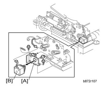
3. DF transport motor with bracket [A] ( otin x 2, spring x 1, timing belt)
