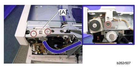
3. Remove the right platen stay holder [A] (  $\ensuremath{\widetilde{F}} \times 3$  ).
