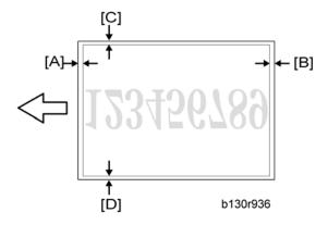
2. Measure the distance between the four edges of the image area and the four edges of the paper [A] [B][C][D].
