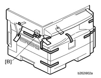
3. Remove the spacing wedge [B].
