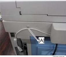
12. Attach the cable clamp [A] to the upper left cover (  $\mathscr{F}$  x 1) as shown above.
