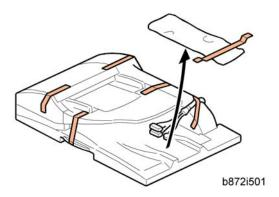
1. Unpack the ARDF and remove the packing tape from the bottom of the ARDF body.
