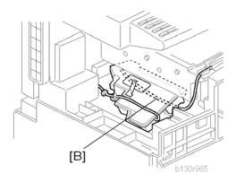
Make sure that the cable [B] passes under the unit.
