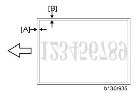
4. Measure the distance between the leading edge of the image area and the leading edge of the paper [A].
