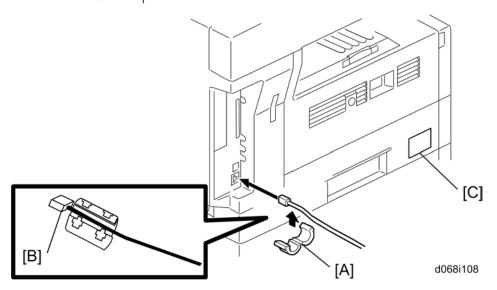
17. Attach the ferrite core [A] to the network cable and attach the cable to the copier if a network cable is used.
