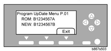
firmware. "NEW" is the information on the firmware in the SD card.
