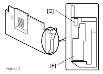
6. Cut the opening [F] on the rear cover. This opening is for the network interfaces and the SD card slot and the LAN cable.
