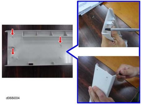
6. Make three holes in the upper left cover with a screwdriver as shown above.
