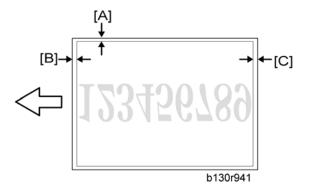
4. Measure the distance between the side edge of the image area and the side edge of the paper [A].
