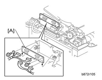
2. DF drive board [A] ( x 2, v x 4, ground cable x 1)
