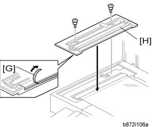
6. Peel off the backing [G] of the double-sided tape attached to the rear side of the left scale guide [H], then install it (F x 2 removed in step 4).
