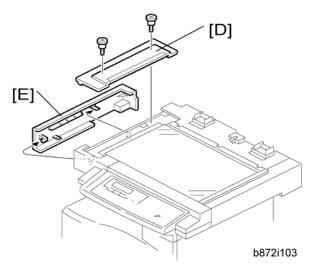
4. Remove the left guide [D] ( $\mathscr{F}$  x 2) and scanner left cover [E] (hook x 2).
