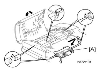
2. Original feed unit [A] ( $\langle \overline{\langle} \rangle \times 1$ )
