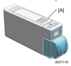
17. Attach the decal [A] to the USB2.0/SD Slot as shown above.
