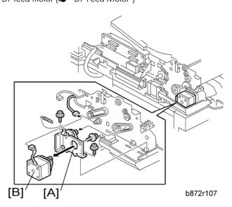
3. DF transport motor with bracket [A] (  $\mathscr{F} \times 2$ , spring x 1, timing belt)
