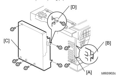
7. Install the ground plate [A] ( $\mathscr{F} \times 2$ ).
