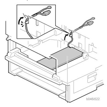
23. Pull the excess length of the heater's harness out the opening at the rear.
