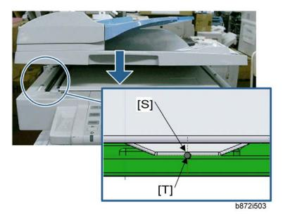
20. Check that the groove [S] of the ARDF is aligned with the groove [T] of the left scale on the scanner.
