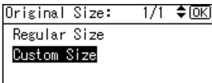
5. Enter the horizontal size of the original (Horiz.) with the number keys, and then press the [OK] key.
