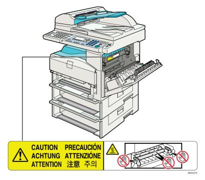
High temperature. Be careful of hot parts when clearing paper jams.
