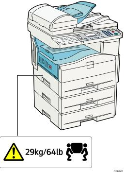
The machine weighs approximately 29 kg (64.0 lb.). When moving the machine, use the inset grips on both sides, and lift slowly in pairs.
