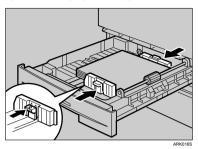
**2** While pinching the release levers, set the end fence to the new paper size.
