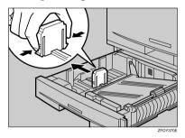
To load  $8^{1}/_{4}$ "×14" $\square$  or  $8^{1}/_{2}$ "×14" $\square$  size paper: pull the end fence out of the tray and place it in the corner pocket on the left.
