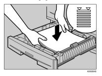
While pressing the release levers, push in the side and end fences until they are flush against the paper's edges.
