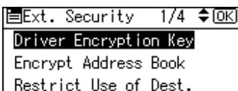
**6** Enter the driver encryption key, and then press the **[OK]** key.
