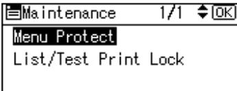
**5** Select the menu protect level using [▲] or [▼], and then press [OK] key.
