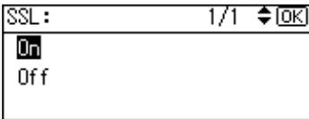
If you do not use secure sockets layer (SSL) for authentication, press [Off].
