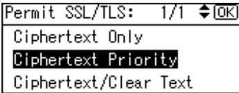
Select **[Ciphertext Only]**, **[Ciphertext Priority]**, or **[Ciphertext/Clear Text]** as the encrypted communication mode.
