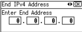
Be sure the number you enter for End IPv4 Address is larger than that for Start IPv4 Address.
