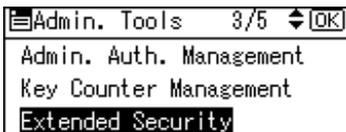
**5** Select [Driver Encryption Key] using [▲] or [▼], and then press the [OK] key.
