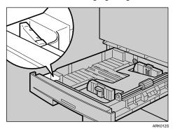
**5** While pressing the release lever, slide the side fences outward.
