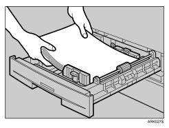
Check that the top of the stack is not higher than the limit mark inside the tray.
