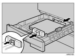
**9** While pinching the release levers, set the end fence to the new paper size.
