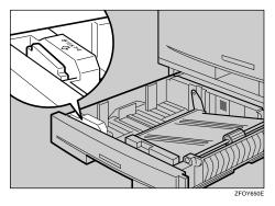
**5** While pressing the release lever, slide the side fence outward.
