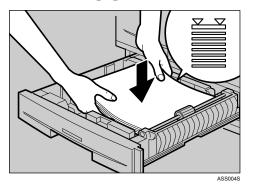
**2** While pressing the release levers, push in the side and end fences until they are flush against the paper's edges.
