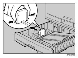
To load  $8^1/4"\times 14"\Box$  or  $8^1/2"\times 14"\Box$  size paper: pull the end fence out of the tray and place it in the corner pocket on the left.
