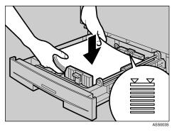
**2** While pressing the release lever, push in the side fences until they are flush against the paper's edges.
