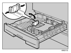
To load A4 $\square$  size paper: place the end fence in the corner pocket on the left.
