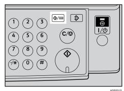
**2** Select [System Settings] using [▼] or [▲], and then press the [OK] key.
