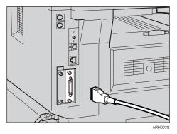
Connect the other end of the cable into the interface connector on the host computer.
