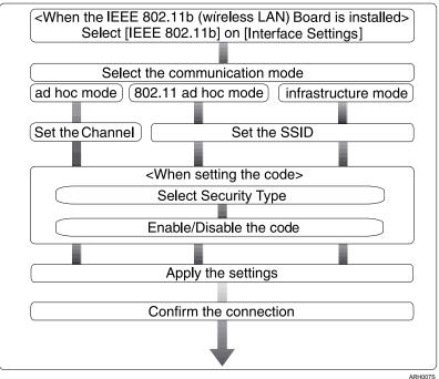
■ IEEE 802.11b (wireless LAN) setup procedure
