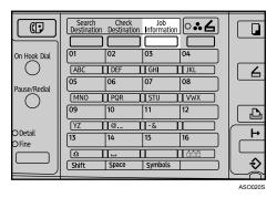
**2** Select [RX File Status] using [▲] or [▼], and then press the [OK] key.
