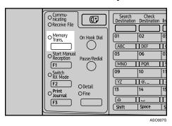
If Memory Trans. indicator is lit, press the **[Transmission Mode]** key to select Immediate Transmission mode.
