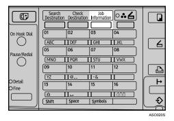
**2** Select [Print TX Standby File] using [▲] or [▼], and then press the [OK] key.
