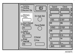
Check the indicator on the operation panel to see which mode is currently active. If it is not lit, Immediate Transmission mode is set.
