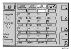
**3** Select [Print Memory Lock File] using [▲] or [▼], and then press the [OK] key.
