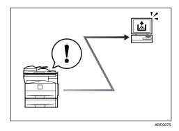
Web Image Monitor lets you configure and operate the machine using a Web browser on a computer. You can also install SmartDeviceMonitor for Admin on a computer to configure and operate the machine.
