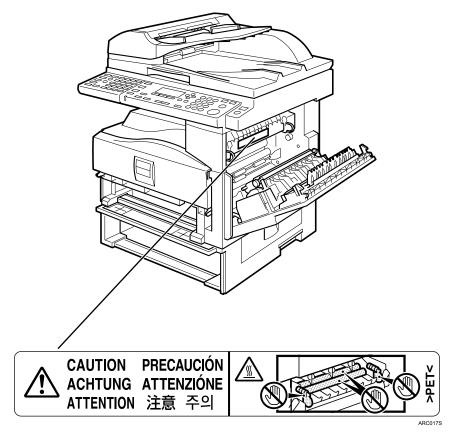
High temperature. Be careful of hot parts when clearing paper jams.
