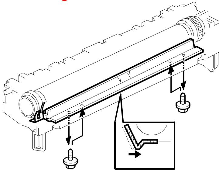
If the paper creases in the fusing unit, move the guide to the right.
