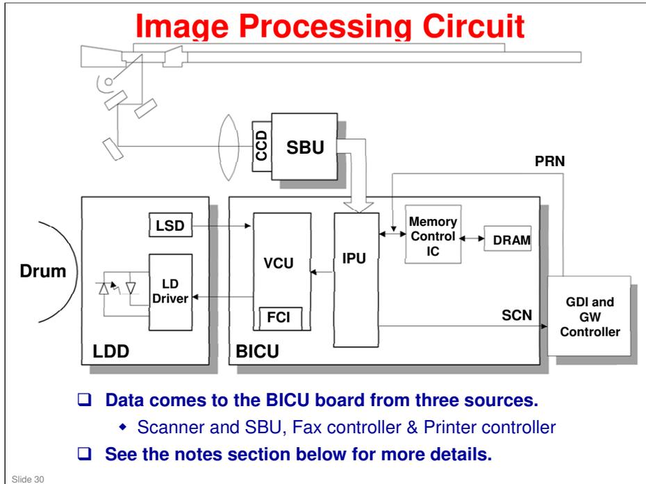
The CCD generates an analog video signal. The SBU (Sensor Board Unit) converts the analog signal to an 8-bit digital signal, then it sends the digital signal to the BICU board. The BICU board can be divided into three image-processing blocks: the IPU (Image Processing Unit), FCI (Fine Character Image), and VCU (Video Control Unit).
