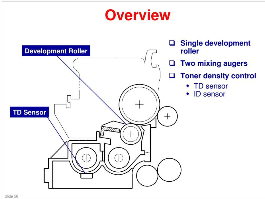
This machine uses a single-roller development system. Two mixing augers mix the developer. The toner density (TD) sensor and image density (ID) sensor (see the illustration in the PCU section) are used to control the image density.
