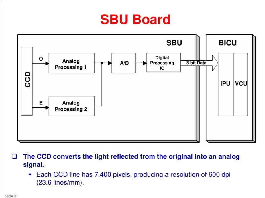
The CCD converts the light reflected from the original into an analog signal. The CCD line has 7,400 pixels and the resolution is 600 dpi (23.6 lines/mm).
