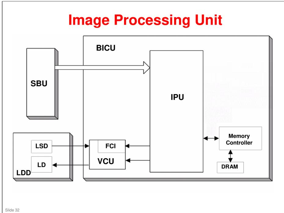
The image data from the SBU goes to the IPU (Image Processing Unit) on the BICU board, which carries out the following processes on the image data:
