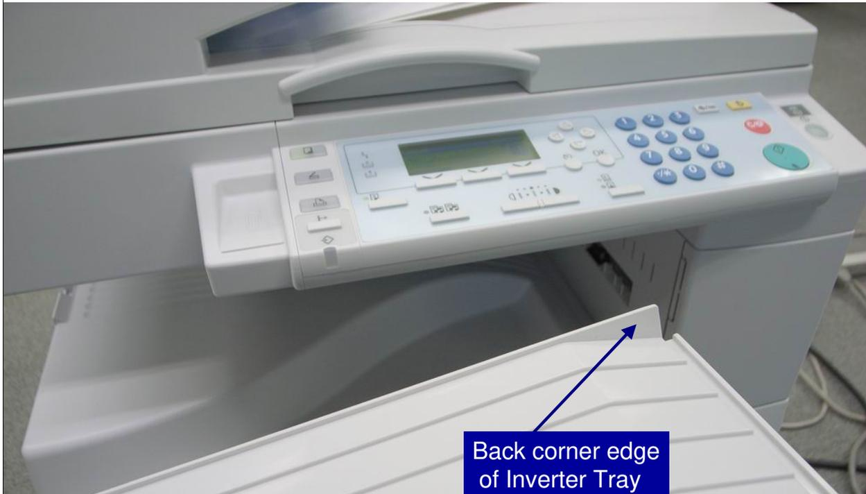
**Check that the back corner edge of the Inverter tray is fully against the back of the slot (see following slides for details).**
