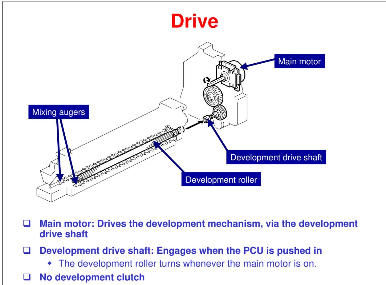
The main motor drives the development roller and mixing augers through a train of gears and the development drive shaft. When the PCU is pushed in, the development drive shaft engages the development roller gear.
