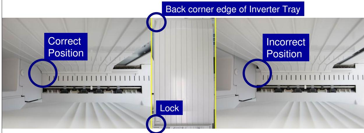
Insure that the back corner edge of the Inverter Tray is fully against the back of the slot. If the back corner edge is away from the back (see right photo above), then duplex printing will jam (see next slide), due to paper hitting the corner edge (see previous slide).
