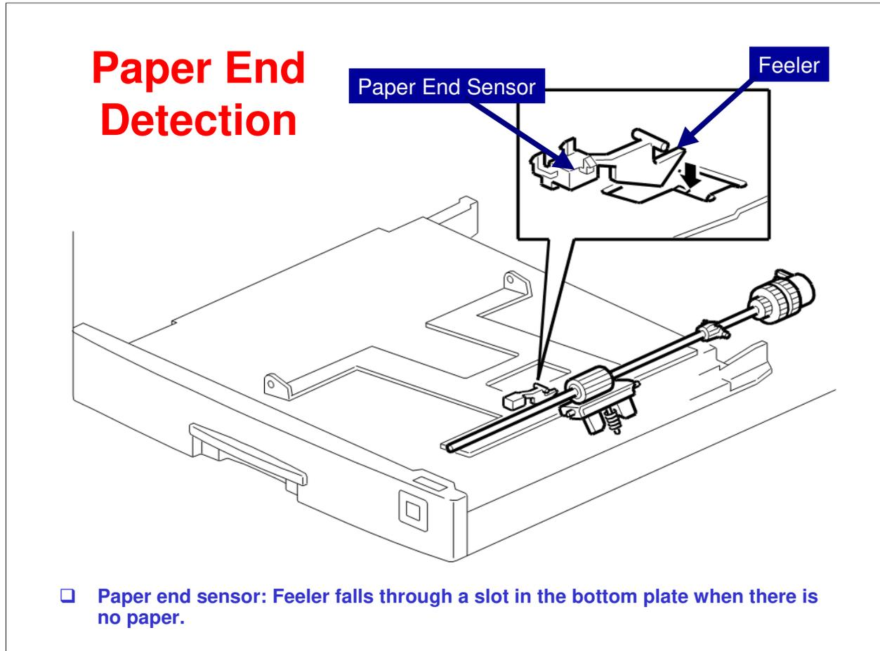
The paper end sensor is mounted on the frame above the paper tray. If there is any paper in the paper tray, the paper stack lifts the feeler and the paper end sensor is deactivated.
