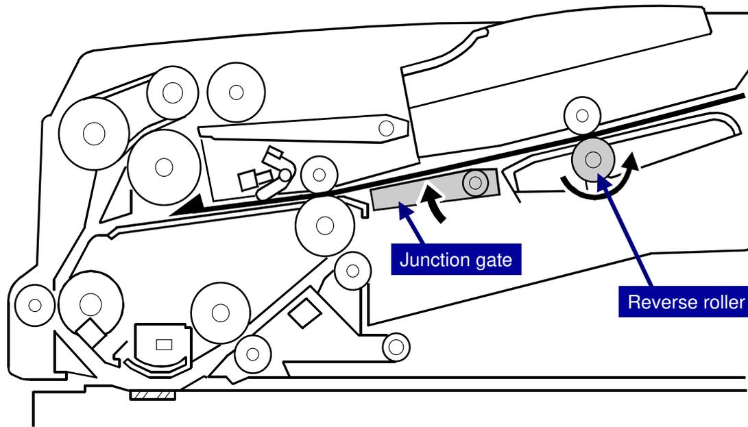
When the paper is in the reverse tray, the junction gate closes. The DF feed motor reverses and the reverse roller feeds the original back into the ARDF.
