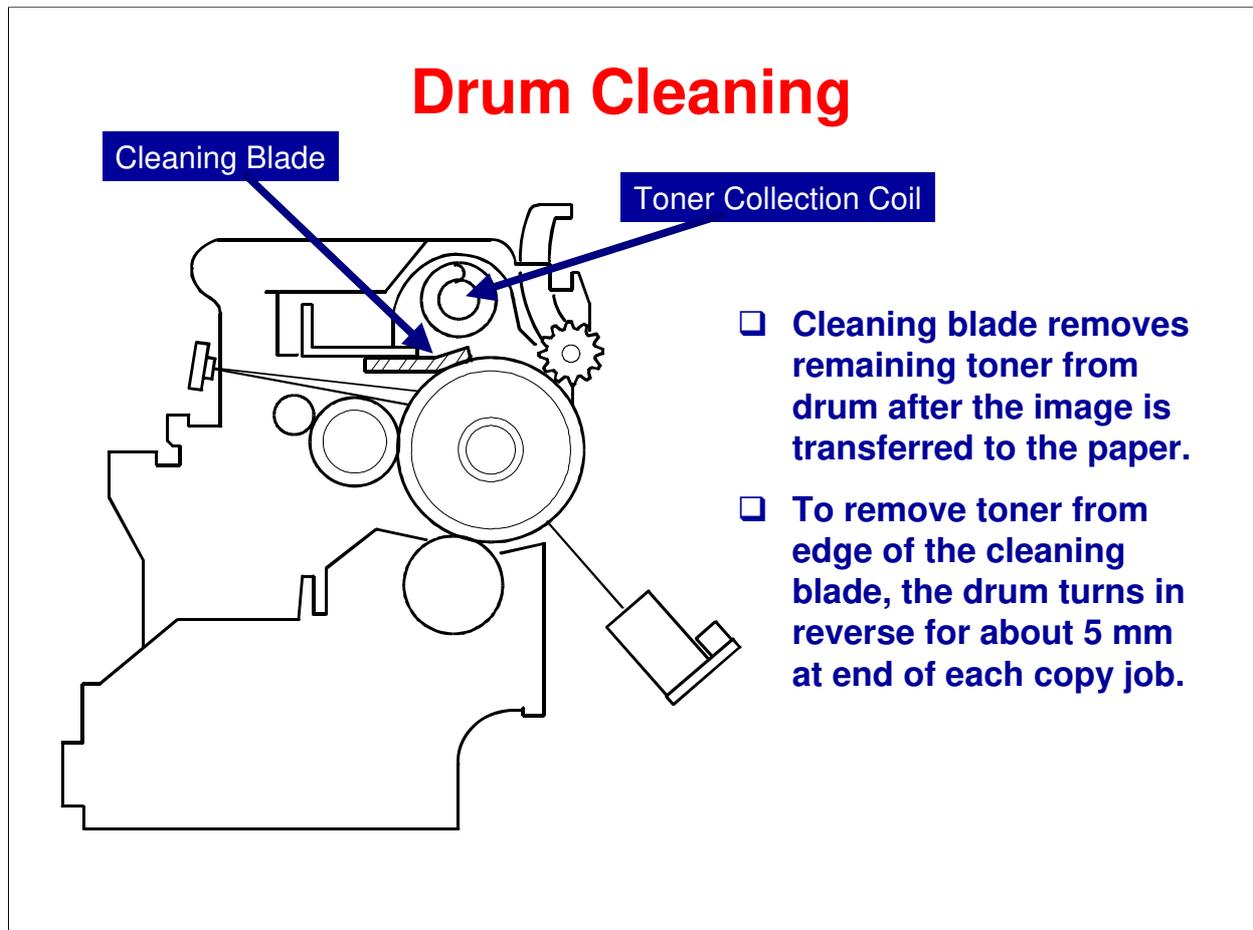
The cleaning blade removes any toner remaining on the drum after the image is transferred to the paper. This model uses a counter blade system. (See the Core Technology Manual for more information on cleaning systems.)
