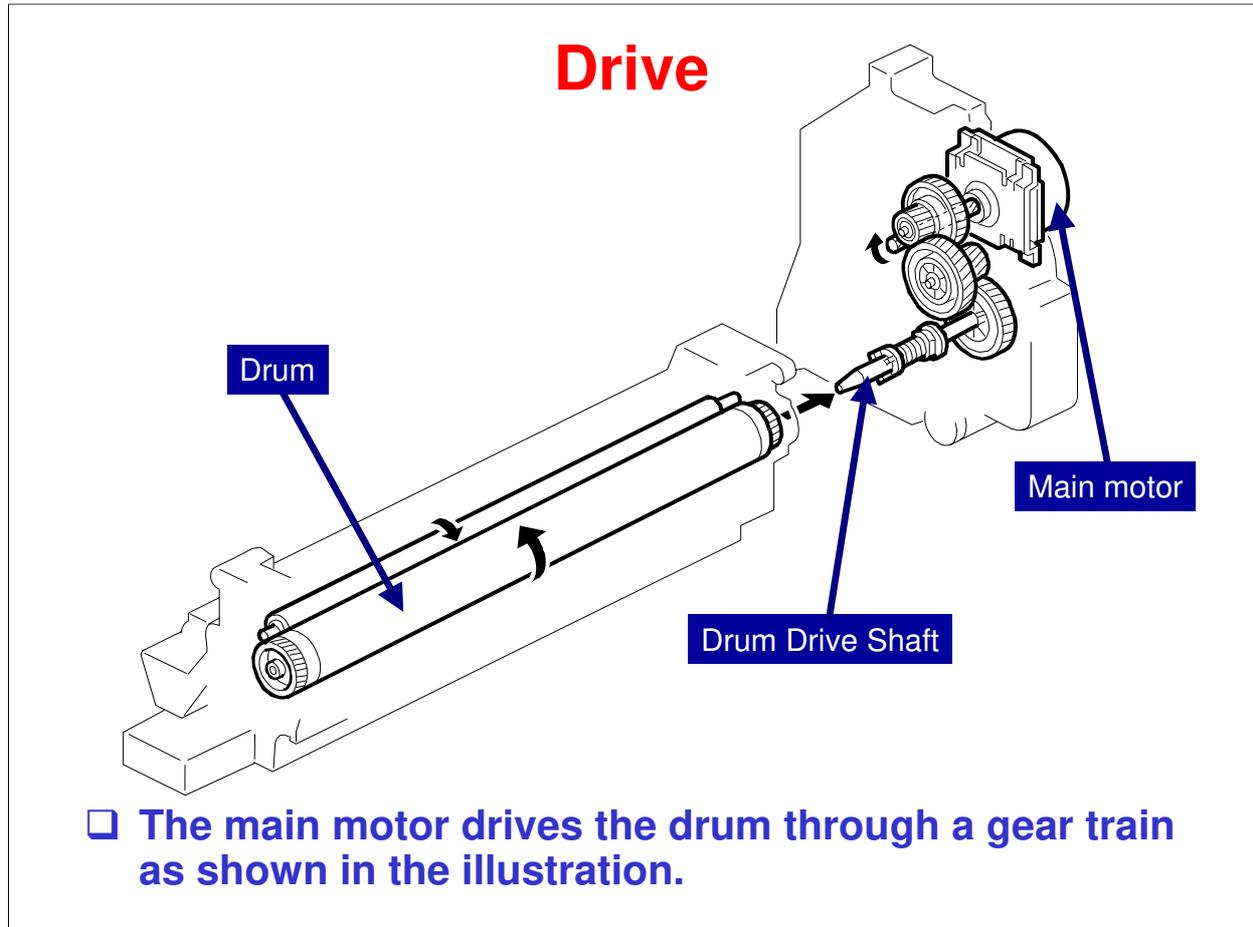
The main motor drives the drum through a series of gears and the drum drive shaft. The main motor assembly includes a drive controller, which outputs a motor lock signal when the rotation speed is out of the specified range.
