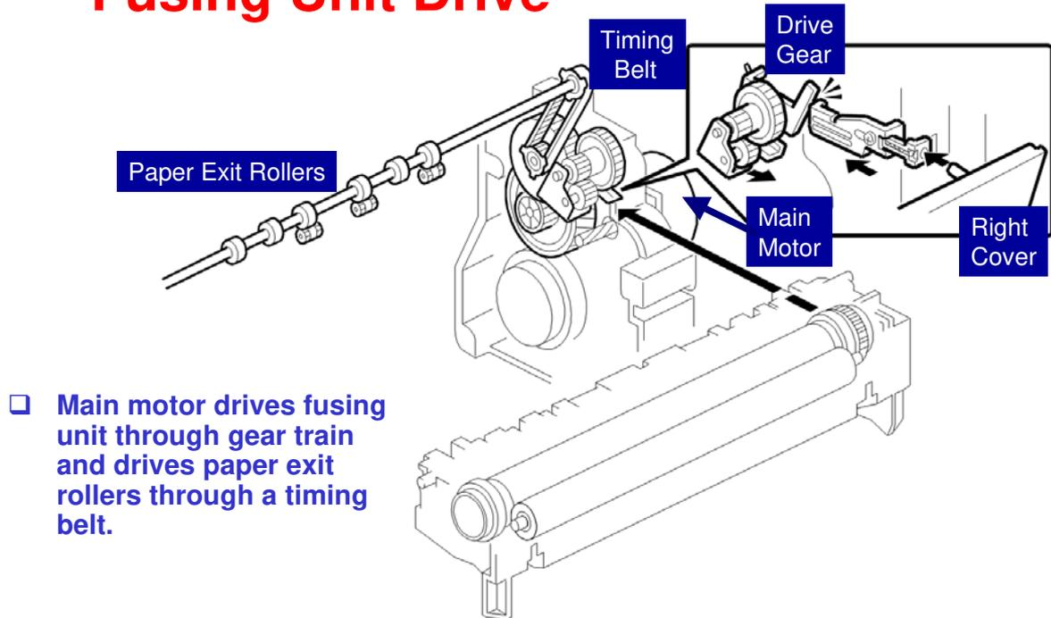
□ Main motor drives fusing unit through gear train and drives paper exit rollers through a timing belt.
