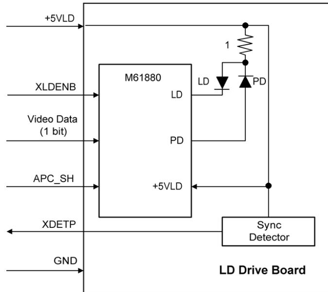
The LD driver IC drives the laser diode. To prevent the intensity of the laser beam from changing because of the temperature, the machine monitors the current passing through the laser diode (LD). The machine adjusts the current to the laser diode by comparing it with the reference level from the reference circuit.
