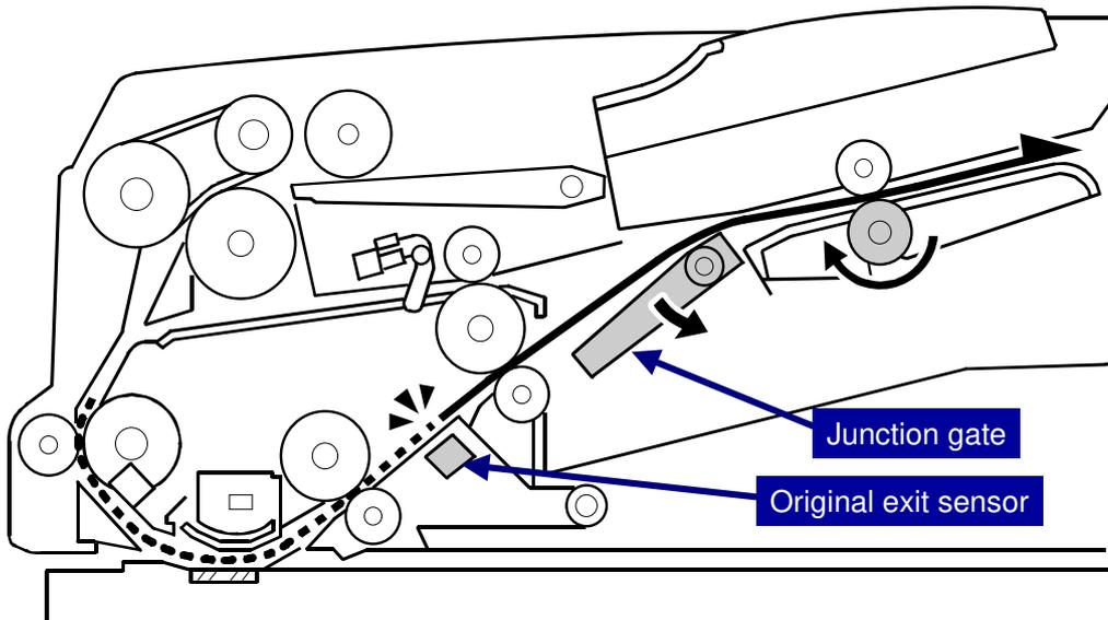
When the original exit sensor detects the leading edge, the junction gate opens and the original goes to the reverse tray.
