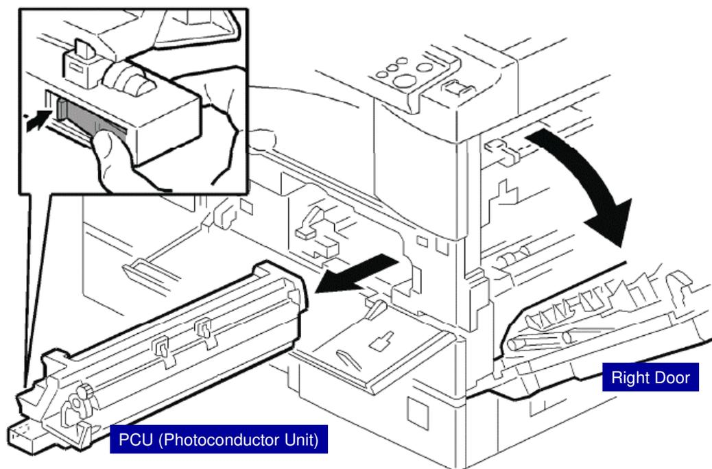
Open the Right Door and remove the PCU (Photoconductor Unit)
