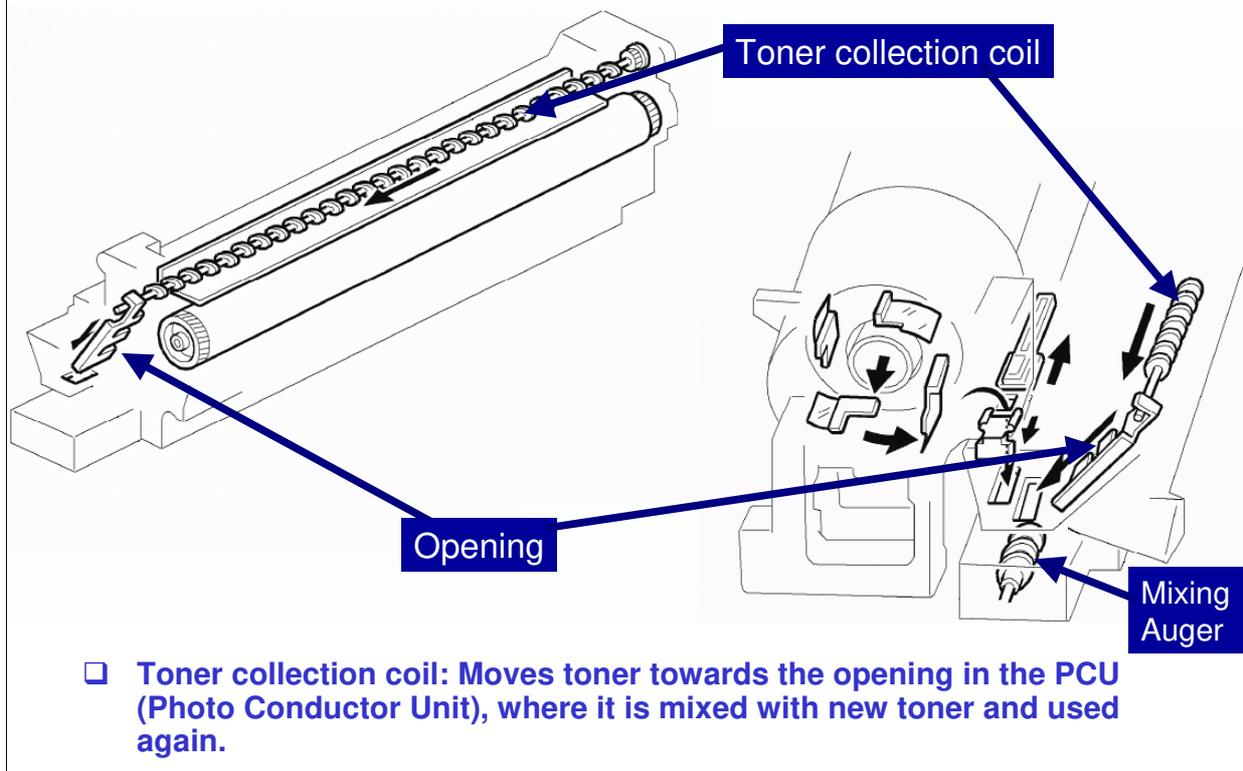
Toner picked up by the toner collection coil, is transported to the opening in the side of the PCU. This toner falls into the development unit with new toner coming from the toner bottle and it is all mixed together in the developer by the mixing auger.
