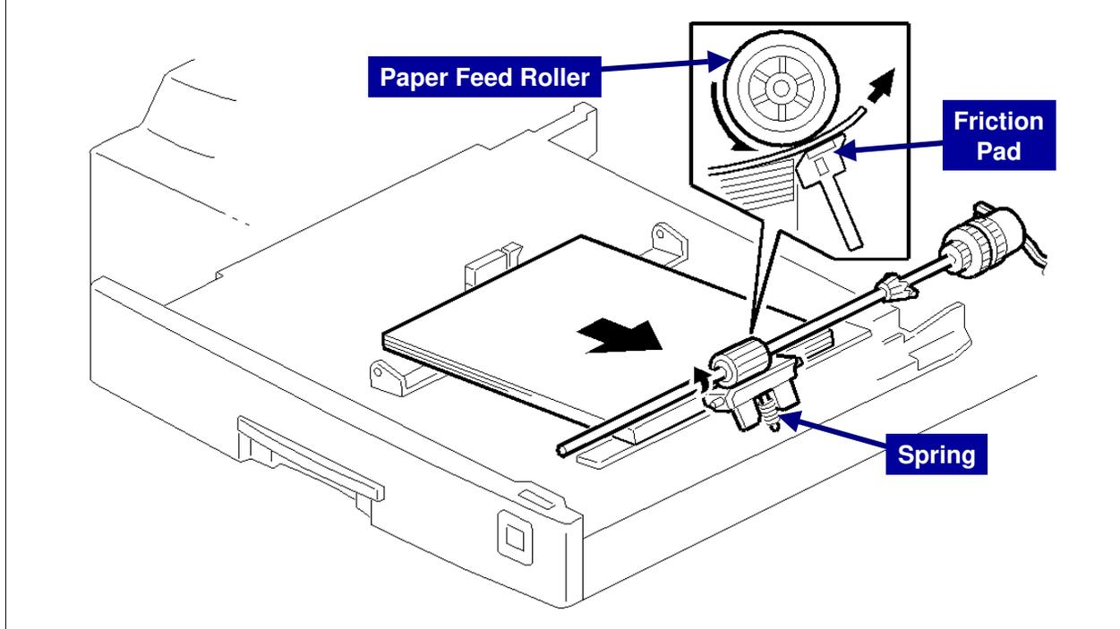
The paper feed roller drives the top sheet of paper from the paper tray to the copier. The friction pad allows only one sheet to feed at a time. The friction pad is pressed against the feed roller by a spring.
