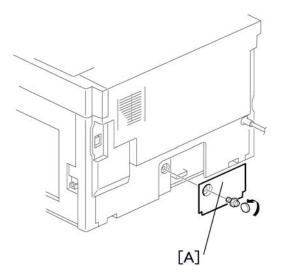
2. Remove the cover [A] (1 rivet).
