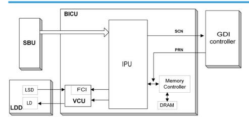
The image data from the SBU goes to the IPU (Image Processing Unit) on the BICU board, which carries out the following processes on the image data:
