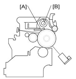
The cleaning blade [A] removes any toner remaining on the drum after the image is transferred to the paper. This model uses a counter blade system.
