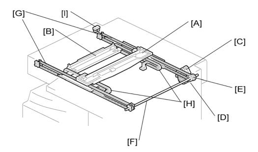
A stepper motor drives the 1st and 2nd scanners [A, B]. The 1st scanner is driven by the scanner drive motor [C], drive gear through the timing belt [D], scanner drive pulley [E], scanner drive shaft [F], and two timing belts [G]. The 2nd scanner is driven through the 1st scanner and two timing belts [H].
