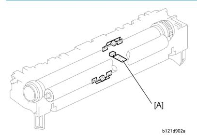
There are the fusing lamp, the thermistor [A], and two thermostats.
