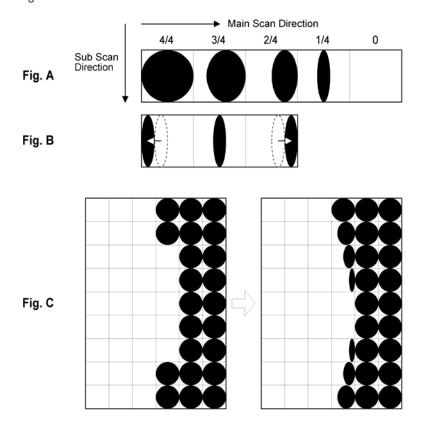
Usually, binary picture processing generates jagged edges on characters, as shown in the above illustration. These are reduced using edge smoothing. The FCI changes the laser pulse duration and position for certain pixels.
