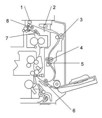
The printed page from the fusing unit goes straight through to the exit tray, or upward to the inverter section, depending on the position of the junction gate.
