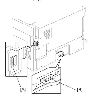
[A]: Socket for ADF/ARDF (Rated voltage output max. DC24 V)
