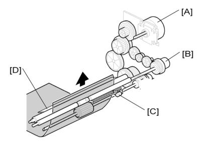
The drive from the main motor [A] is transmitted to the registration roller through the registration clutch gear [B].
