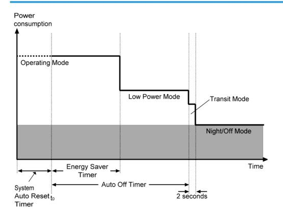
The machine has three energy-saver modes: the Low Power Mode, the Transit Mode, and the Night/Off Mode. The Transit Mode continues for about two seconds (probably, the user does not recognize this mode when it occurs). The table lists the status of several components. For the fusing temperature, see the section of "Fusing Temperature Control".
