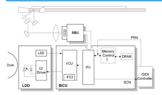
The CCD generates an analog video signal. The SBU (Sensor Board Unit) converts the analog signal to an 8-bit digital signal, then it sends the digital signal to the BICU board.
