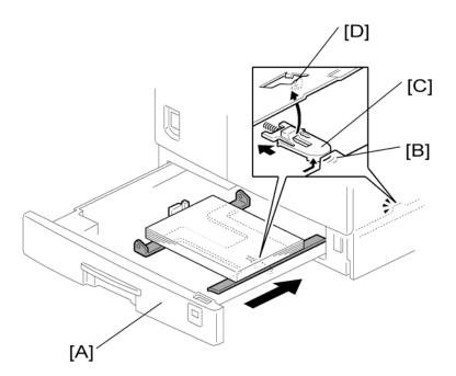
When the paper tray [A] is closed, projection [B] on the copier frame pushes slider [C] (on the bottom part of the paper tray) off the bottom plate hook [D]. After the release slide comes off, compressed springs lift the bottom plate.
