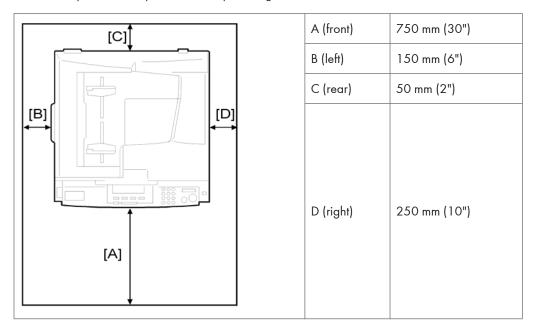
The recommended 750 mm front space is sufficient to allow the paper tray to be pulled out. Additional front space is required to allow operators to stand at the front of the machine.
