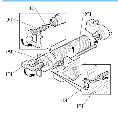
When a toner bottle is placed in the bottle holder unit [A] and the unit is pushed in completely, toner shutter [B] moves against the side [C] of the PCU. When the toner bottle holder lever [D] is put back in the original position, the cap [E] on the toner bottle is pulled away and kept in place by the chuck [F].
