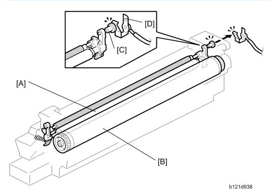
This copier uses a drum charge roller to charge the drum. The drum charge roller [A] always contacts the surface of the drum [B] to give it a negative charge of -950 V. The high voltage supply board gives a negative charge of -1700 V to the drum charge roller through the screw [C] and terminal plate [D]. This voltage can be changed using SP 2001 1.
