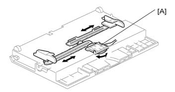
The by-pass feed paper size switch [A] monitors the paper width. The side fence is connected to the terminal plate gear. When the side fences move to match the paper width, the circular terminal plate rotates over
