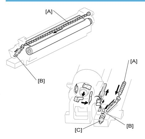
Toner picked up by the toner collection coil [A], is transported to the opening [B] in the side of the PCU. Then, this toner falls into the development unit with new toner coming from the toner bottle and it is all mixed together by mixing auger 1 [C] and used again.
