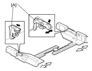
If the tray is full of paper and it is pushed in strongly, the fences may deform or bend. This may cause the paper to skew or the side-to-side registration to be incorrect. To correct this, each side fence has a stopper [A] attached to it. Each side fence can be secured with a screw, for customers who do not want to change the paper size.
