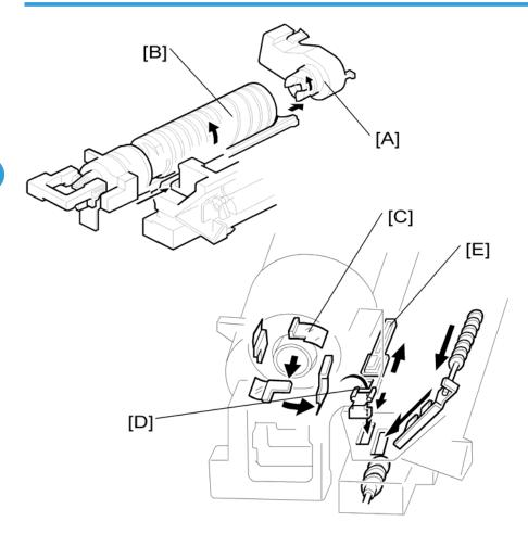
The toner supply motor [A] drives the toner bottle [B] and the mylar blades [C]. First, the toner falls down into the toner bottle holder. The toner supply mylar blades transfer the toner to the slit [D]. When the PCU is installed in the machine, the shutter [E] above the PCU is opened by the toner bottle holder. Then the toner falls down into the development unit through the slit and the shutter.
