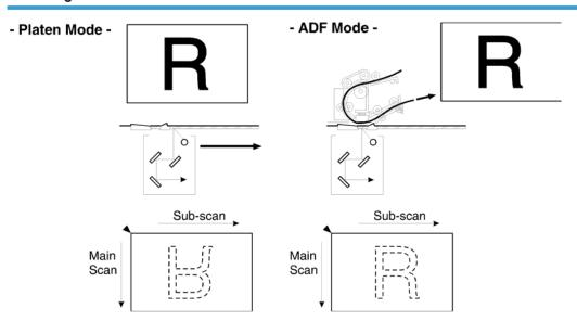
When making copies using the ADF, the magnification circuit creates a mirror image. This is because the scanning start position along the main scan direction in ADF mode is at the opposite corner of platen mode.
