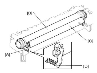
The pressure springs [A] constantly apply pressure between the hot roller [B] and the pressure roller [C]. Applied pressure can be changed by adjusting the position of the pressure springs. The spring is positioned at the end [D] as the default setting.
