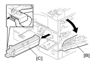
3. Open the right door [B], and remove the PCU (photoconductor unit) [C].
