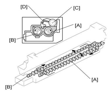
The two mixing augers, [A, B] keep the developer evenly mixed. Mixing auger 2 [A] transports excess developer, scraped off the development roller [C] by the doctor blade [D], towards the front of the machine. Mixing auger 1 [B] returns the excess developer, along with new toner, to the rear of the mixing assembly. Here the developer is reapplied to the development roller.
