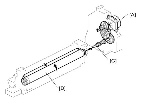
The main motor [A] drives the drum [B] through a series of gears and the drum drive shaft [C]. The main motor assembly includes a drive controller, which outputs a motor lock signal when the rotation speed is out of the specified range.
