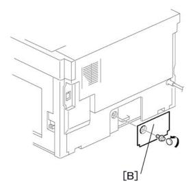
3. Remove the cover [B] (1 rivet).
