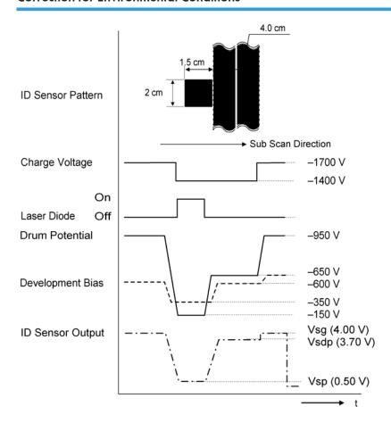
With a drum charge roller system, the voltage transferred from roller to drum varies with the temperature and humidity around the drum charge roller. The higher the temperature or humidity is the higher the applied voltage required.
