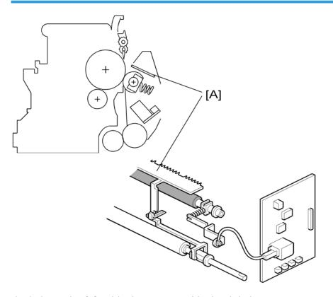
The discharge plate [A] and the drum curvature of the drum help the paper to separate away from the drum. The discharge plate is grounded.
