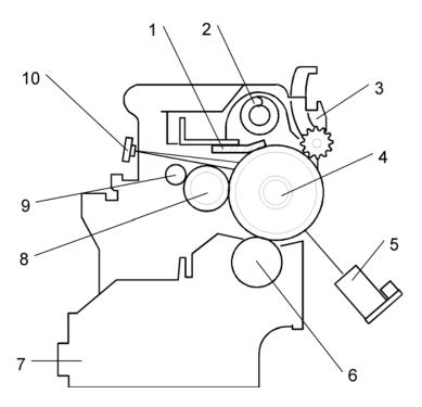
The PCU consists of the components shown in the above illustration. An organic photoconductor (OPC) drum (diameter: 30 mm) is used in this machine.
