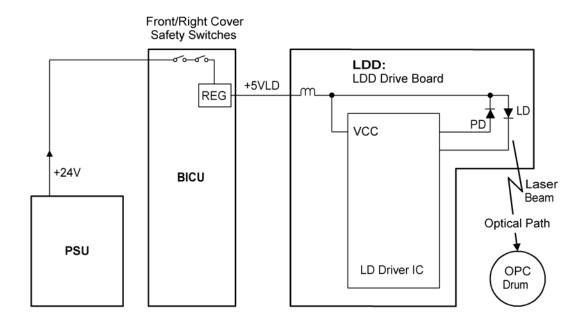
To ensure technician and user safety and to prevent the laser beam from inadvertently switching on during servicing, there are safety switches at the front and right covers.
