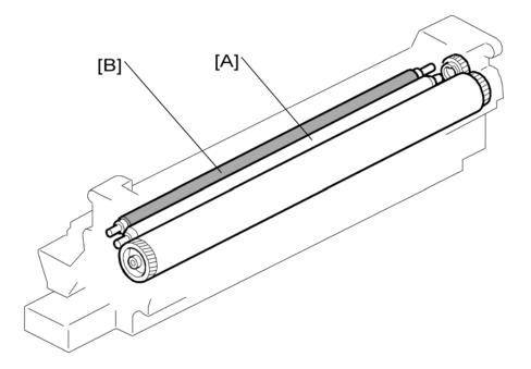
Because the drum charge roller [A] always contacts the drum, it gets dirty easily. So, the cleaning brush [B] also contacts the drum charge roller all the time to clean the surface of the drum charge roller.
