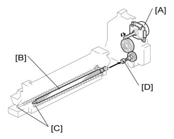
The main motor [A] drives the development roller [B] and mixing augers [C] through a train of gears and the development drive shaft [D]. When the PCU is pushed in, the development drive shaft engages the development roller gear.
