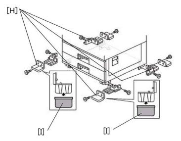
11. Install the four brackets with long supports [H] and covers [I] (2 screws each).
