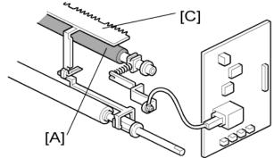
The transfer roller [A] touches the surface of the drum [B]. The high voltage supply board supplies a positive current to the transfer roller, which attracts the toner from the drum onto the paper. The current depends on the paper width, paper type, and paper feed tray.
