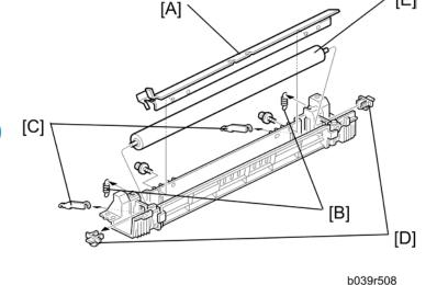
1. Separate the fusing unit into two sections: the hot roller section and the pressure roller section (
