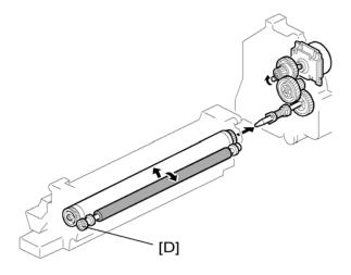
Drive from the drum through a gear [D] turns the transfer roller.
