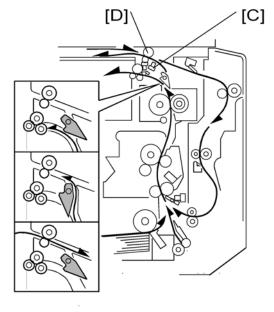
During duplex copying, the inverter gate solenoid [A] switches on and the junction gate [B] switches over to direct the paper to the inverter. When the paper trailing edge reaches the duplex inverter sensor [C], the inverter roller [D] reverses its rotation direction and the paper goes to the duplex unit. The paper is then sent to the mainframe registration rollers to print the reverse side.
