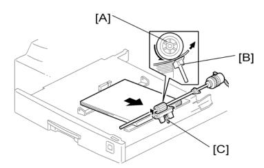
The paper feed roller [A] drives the top sheet of paper from the paper tray to the copier. The friction pad [B] allows only one sheet to feed at a time. The friction pad applies pressure to the feed roller with a spring [C].
