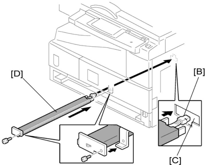
3. Pass the connector [B] through the opening [C] and install the tray heater [D] (⌀ x 1).
