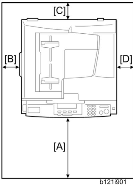
The recommended 750 mm front space is sufficient to allow the paper tray to be pulled out. Additional front space is required to allow operators to stand at the front of the machine.
