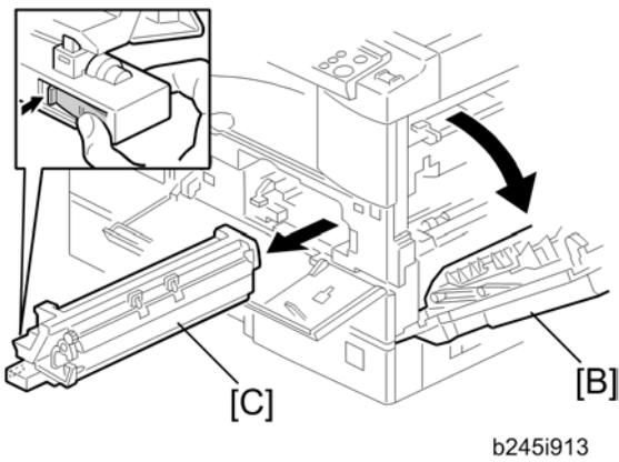
3. Open the right door [B], and remove the PCU (photoconductor unit) [C].
