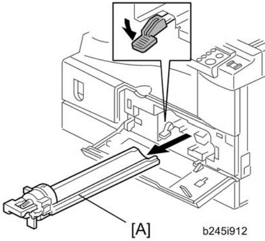
2. Open the front door and remove the toner bottle holder [A]
