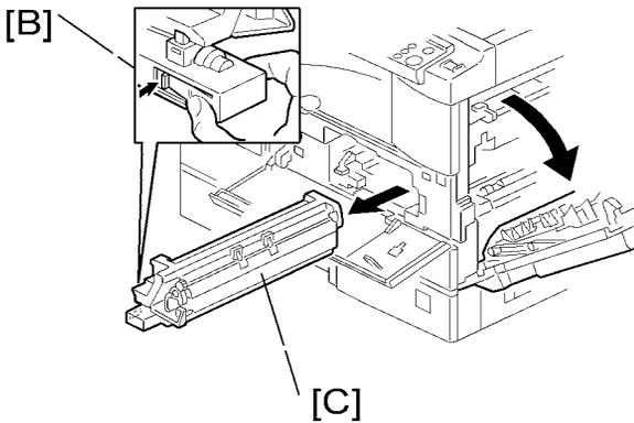
3. Press the latch [B] and pull out the PCU [C].
