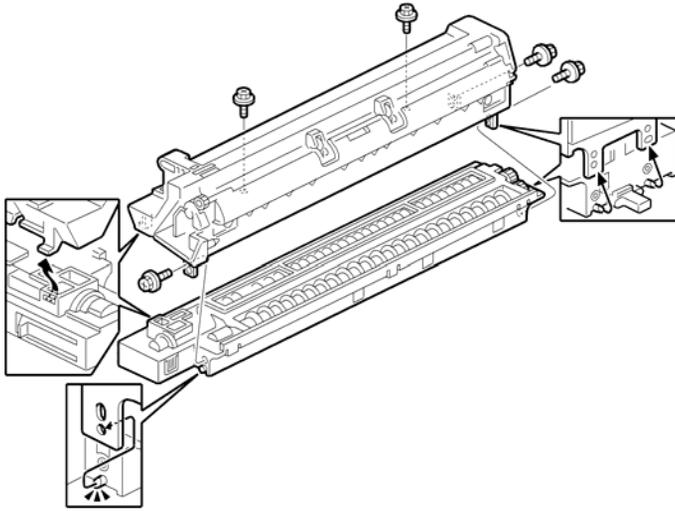
4. Separate the PCU into the upper part and the lower part (⚙ x 5).
