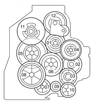
The gears are numbered 1 to 12 in the order in which they are to be installed in the gearbox. These numbers show both on the gearbox and on the front (exposed) surface of each gear. If the gears fall out, start by finding gear number 1 and installing it onto location number 1 (setting it into place so that the side with the printed number stays visible). Then install the remaining gears (2 to 12) in the same way.
