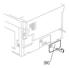
3. Remove the cover [B] (1 rivet).
