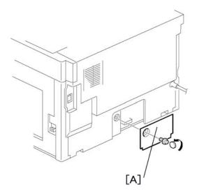
2. Remove the cover [A] (1 rivet).
