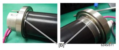
• Apply the "Barrierta S552R" to the hot roller shaft so that the applied grease (white line) [B] comes out between the hot roller shaft and inside of the hot roller bushing.
