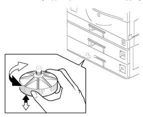
12. Rotate the adjuster (installed at step 2) to fix the machine in place.
