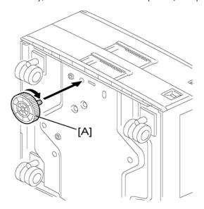
2. Attach the adjuster [A] to the base plate as shown.
