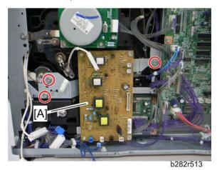
3. High-voltage power supply board bracket [A] ( F x 3)
