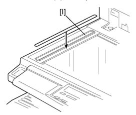
9. Attach the appropriate scale decal [1] as shown.
