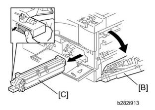
3. Open the right door [B], and remove the PCU (photo conductor unit) [C].
