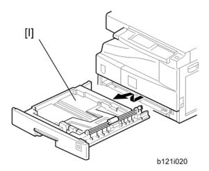
11. Pull out the paper tray [I] and turn the paper size dial to the appropriate size. Adjust the positions of the end and side guides.
