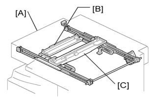
Adjust the scanner positions when the first scanner [C] and second scanner [B] are not parallel with the side frames [A], or, when you have replaced one or more of the scanner belts.
