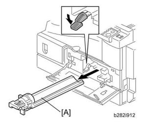
2. Open the front door and remove the toner bottle holder [A].
