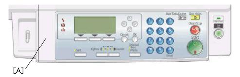
1. Remove the dummy cover [A] from the operation panel
