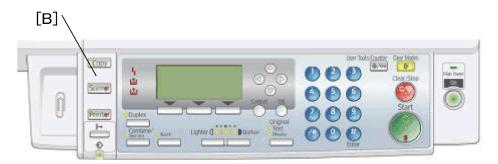
2. Install the printer/scanner panel [B] on the operation panel.
