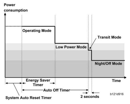
The machine has three energy-saver modes: the Low Power Mode, the Transit Mode, and the Night/Off Mode. The Transit Mode continues for about two seconds (probably, the user does not recognize this mode when it occurs). The table lists the status of several components.
