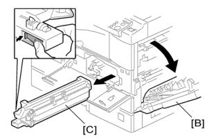
3. Open the right door [B], and remove the PCU (photo-conductor unit) [C].
