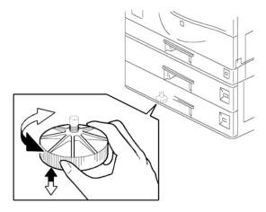
12. Rotate the adjuster (installed at step 2) to fix the machine in place.
