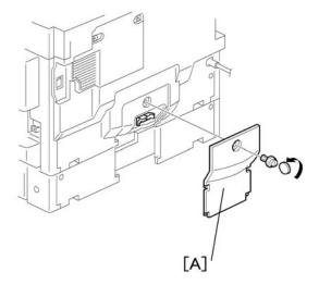
2. Remove the cover [A] (1 rivet).
