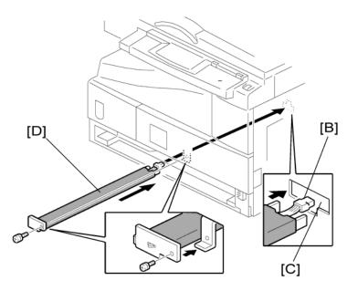
3. Pass the connector [B] through the opening [C] and install the tray heater [D] ( $\nearrow$  x 1).
