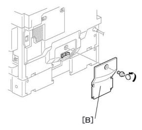
3. Remove the cover [B] (1 rivet).
