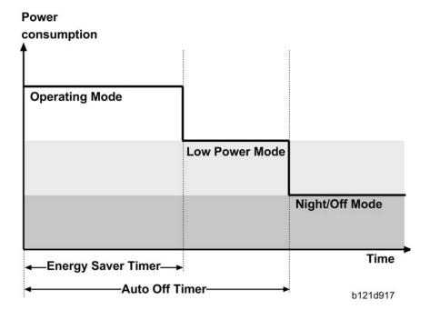
The machine has two energy-saver modes: the Low Power Mode and the Night/Off Mode. The table lists the status of several components.
