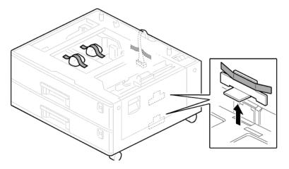
1. Remove the strips of tape. Make sure that you have removed all the strips of tape and all the pieces of cardboard.
