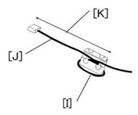
Attach the ferrite core [A] to the network cable [B]. The end of the ferrite core must be about 10 cm (4") from the end of the cable [C].
