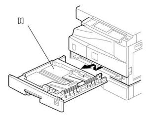
11. Pull out the paper tray [I] and turn the paper size dial to the appropriate size. Adjust the positions of the end and side guides.
