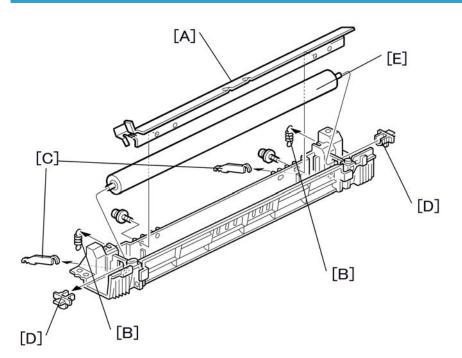
1. Separate the hot roller section from the pressure roller section (\*\* p.123 "Fusing Lamps").
