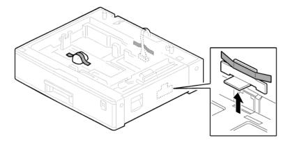
1. Remove the strips of tape. Make sure that you have removed all the strips of tape and all the pieces of cardboard.
