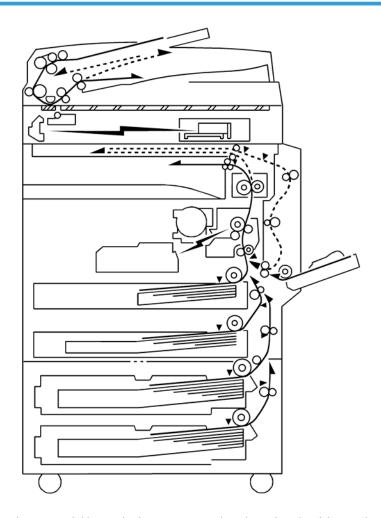
The B244/B269/B277 model has a duplex unit mounted on the right side of the machine. All models have a by-pass tray.
