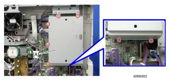
6. Remove the controller box cover [A] ( $\mathscr{F}$  x 7).
