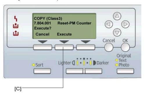
6. To reset the PM counter, press the button [C] below the message "Execute."
