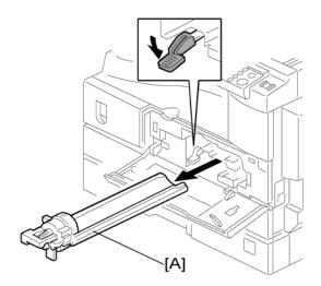
2. Open the front door and remove the toner bottle holder  $\left[ A \right]$
