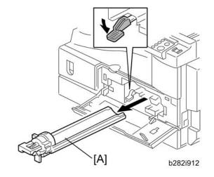
2. Open the front door and remove the toner bottle holder [A].
