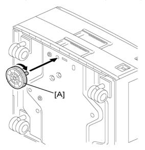
2. Attach the adjuster [A] to the base plate as shown.
