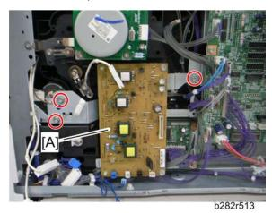
3. High-voltage power supply board bracket [A] ( 🌮 x 3)
