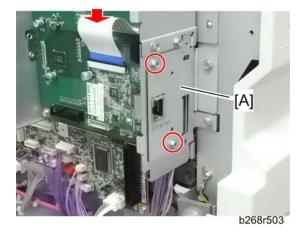
3. NCU [A] if it has been installed ( 🌮 x 2, flat cable x 1)
