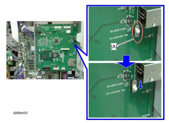
13. Move the switch [A] of the SW2 from "ON" (upper) to "OFF" (lower).
