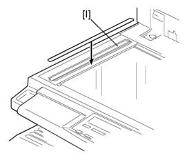
9. Attach the appropriate scale decal [I] as shown.
