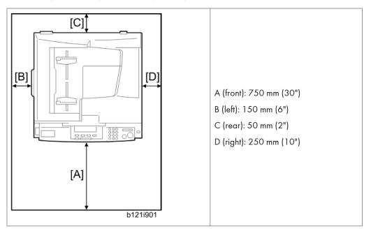
The recommended 750 mm front space is sufficient to allow the paper tray to be pulled out. Additional front space is required to allow operators to stand at the front of the machine.
