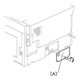
2. Remove the cover [A] (1 rivet).
