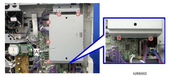
6. Remove the controller box cover [A] (  $\checkmark$  x 7).
