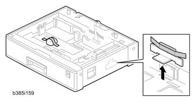
1. Remove the strips of tape. Make sure that you have removed all the strips of tape and all the pieces of cardboard.
