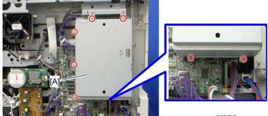
5. Remove the controller box cover [A] (  $\mathscr{P} \times 7$ ).
