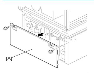
1. Remove the rear cover [A].for the paper tray unit ( 🌶 x 2).
