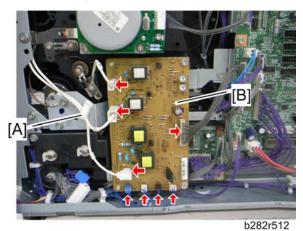
2. Release the clamp [A] and disconnect all connectors on the high-voltage power supply board [B].
