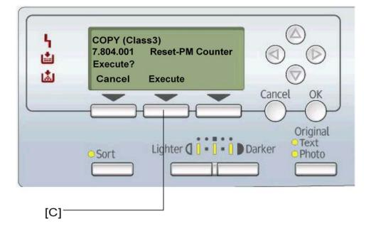
6. To reset the PM counter, press the button [C] below the message "Execute".
