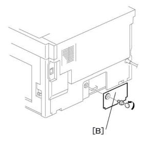
3. Remove the cover [B] (1 rivet).
