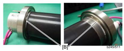
• Apply the "Barrierta S552R" to the hot roller shaft so that the applied grease (white line) [B] comes out between the hot roller shaft and inside of the hot roller bushing.
