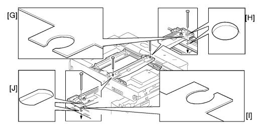
The two actions above have the same objectives--to align the following holes and marks:
