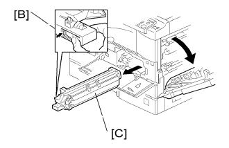
3. Press the latch [B] and pull out the PCU [C].
