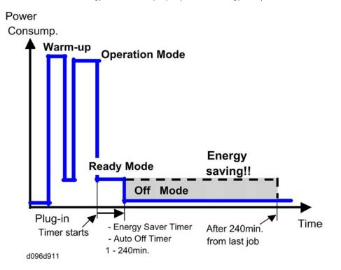
The area shaded grey in this diagram represents the amount of energy that is saved when the timers are at the default settings. If the timers are changed, then the energy saved will be different. For example, if the timers are all set to 240 min., the grey area will disappear, and no energy is saved before 240 min. expires.
