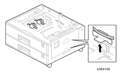
1. Remove the strips of tape. Make sure that you have removed all the strips of tape and all the pieces of cardboard.
