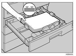
**2** While pressing the release lever, adjust the side and end fences to the new paper size.
