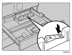
**(U**) While pressing the release lever, slide the side fences outward.
