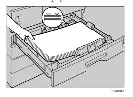
While pressing the release lever, adjust the side and end fences to the new paper size.
