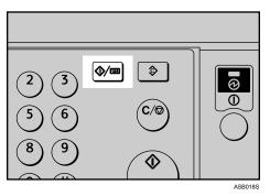
Select [System Settings] using [▲] or [▼], and then press the [OK] key.
