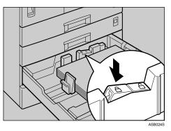
Adjust the paper size selector in the paper tray according to the paper size.
