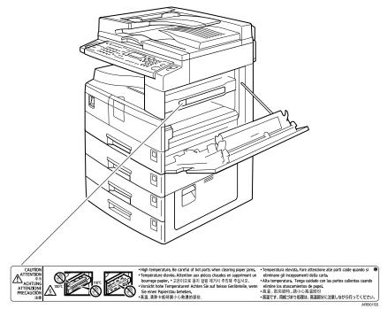
High temperature. Be careful of hot parts when clearing paper jams.
