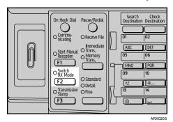
**2** Select the reception mode using [▲] or [▼], and then press the [OK] key.
