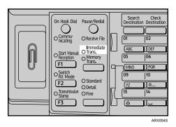
If Memory Trans. indicator is lit, press the **[Transmission Mode]** key to select Immediate Transmission mode.
