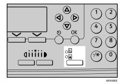
Press the **[Original Type]** key to switch between Text and Photo.
