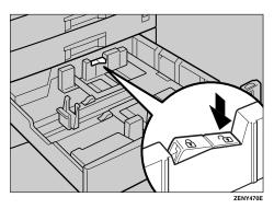
**5** While pressing the release lever, adjust the side fences.
