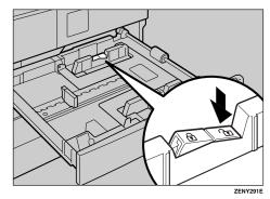
• While pressing the release lever, adjust the side fences.
