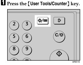
Select [Counter] using [▲] or [▼], and then press the [OK] key.
