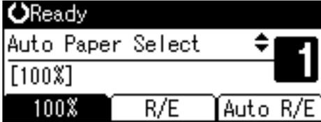
**2** Select [Regular Size] using [▲] or [▼] key, and then press the [OK] key.
