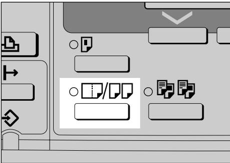
**2** Select the combine mode using [▲] or [▼], and then press the [OK] key.
