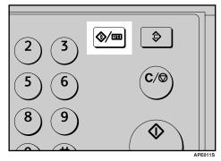
Select [System Settings] or [Copier Features] using [▲] or [▼], and then press the [OK] key.
