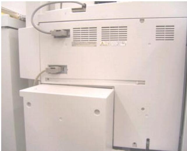
24. Reattach the rear cover and connect the connectors.
