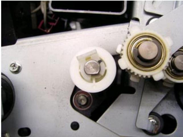
16. Attach the new cleaning drive pulley (1 snap ring).
