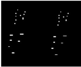
White spots appear as dots or small lines at 314 mm (12 in.) intervals in the direction of paper feed.
