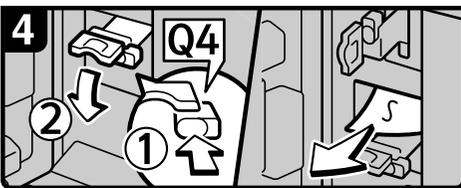
7. Press button Q4, open the guide board.
