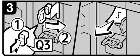
4. Press button Q3, open the guide board.
