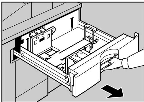
**2** Load paper into the paper tray by pushing the paper to the left side of the paper tray.
