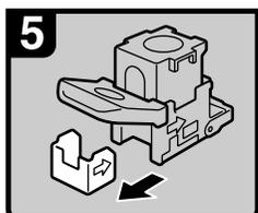
6. Remove the empty refill in the direction of the arrow.
