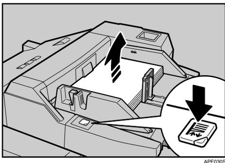
The green lamp of the elevator switch is blinking while the tray is going up and down, and keeps lit when it stops.
