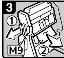
4. Pull handle M9 and pull out staple unit, then remove misfed paper.
