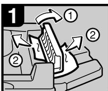
1. Open the cover P2 of the ADF and remove misfed originals.
