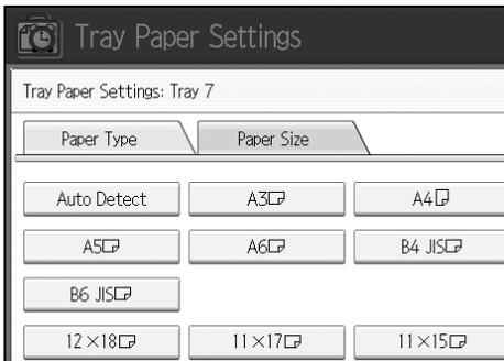
**4** Select a combination of the specified paper size and orientation, and then press **[OK]**.
