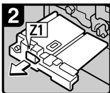
3. Pull handle Z1 and fully pull out the duplex unit.
