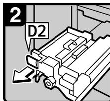
3. Pull lever D2 and fully pull out the fuser unit.
