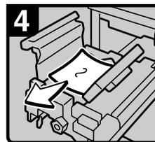
5. Remove misfed paper and return lever D3 and lever D4 to original position.
