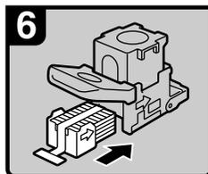
7. Push in the new staples until the arrows are aligned.
