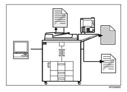
• Using the printer driver, you can embed a pattern in the printed document. If the document is copied on a machine with the Copy Data Security Unit (optional), protected pages are grayed out in the copy, preventing confidential information from being copied. In addition, the machine beeps to notify that unauthorized copying is being attempted.
