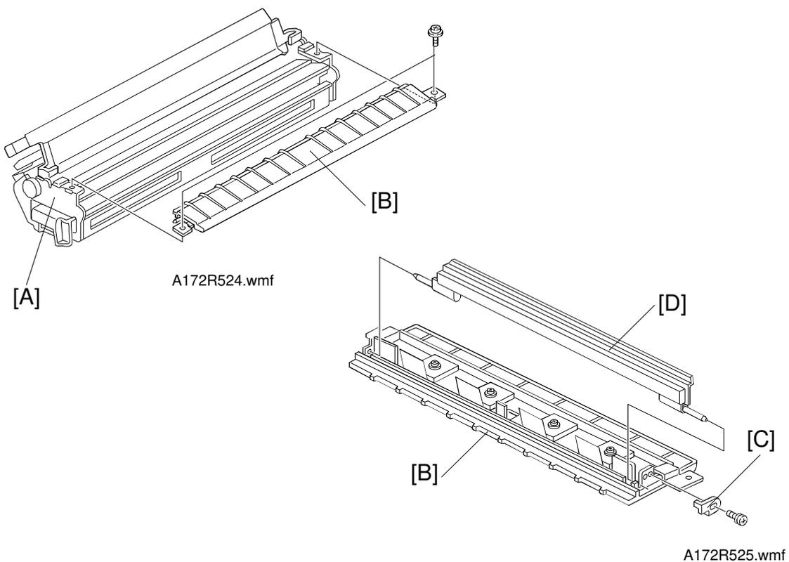
1. Remove the transfer roller unit [A]. (See A109 Transfer Roller Unit Removal).
