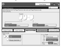
Press the [Image] or [Blank] key depending on whether the reverse side of last original has an image or not.
