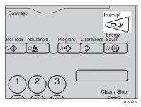
**2** Remove the previous originals. Set your original for interrupt copying on the exposure glass or in the document feeder.
