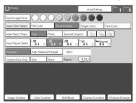
3 Make sure that the [Orig. Horiz.] key is selected. Enter the horizontal size with the number keys, then press the [#] key.
