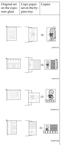
□ If Duplex copying cannot be done because of paper problems, set paper on the bypass tray to copy on the front side, and once again copy on the backside.
