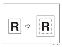
You can move the image to the center. This function is convenient when the copy paper is larger than the original.
