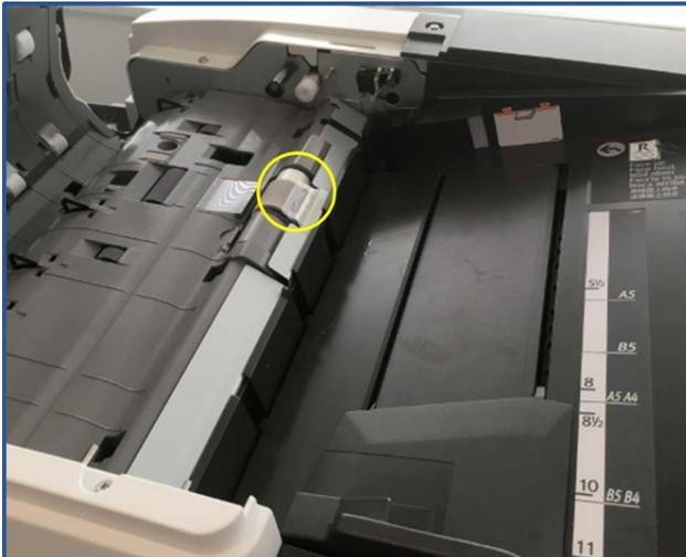
3. Remove the paper feed guide plate.
