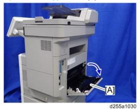
IM 550F/600F only: Insert a flathead screwdriver into [A] to release a hook of the controller cover[B].
