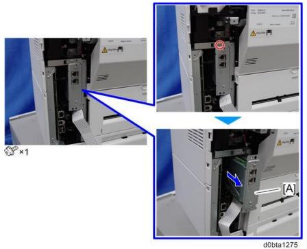
26. Reattach the controller box cover [A].
