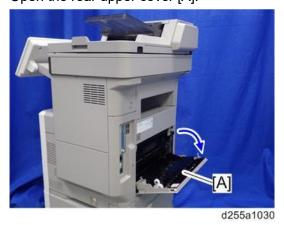
2. IM 550F/600F only: Insert a flathead screwdriver into [A] to release a hook of the controller cover
