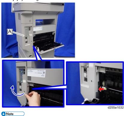
• Be careful not to damage the hooks on the inside of the controller cover when you remove or install the controller cover.
