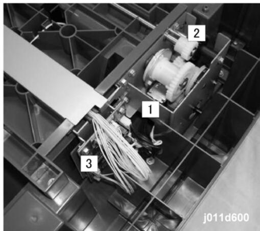
The paper feed motor [1] in the tray drives the feed roller [2]. The control board [3] controls the operation of the feed clutch (not shown). This engages the shaft where the feed roller is mounted. Then it rotates it at the prescribed times to feed paper from the tray.
