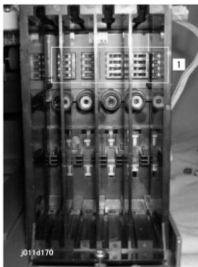
Four micro switches detect the print cartridges. The switches are connected in series above the cartridge set detection plate [1]. Each tank is provided with a micro-switch. The machine can specifically detect which print cartridge is not set correctly. An open switch signals when:
