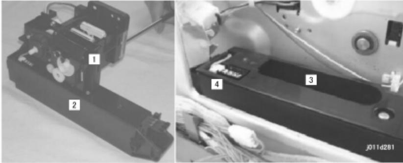
Inside the printer, the maintenance unit [1] sits on top of the ink collector tank [2].
