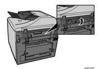
Check the network interface board's orientation, and then install the network interface board gently.
