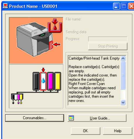
In this illustration, the control panel is indicating that the cyan Print cartridge and Print head tank are empty.
