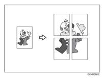
You can enlarge the complete image of originals onto several sheets. This function is convenient for making posters.
