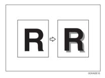
This function adds a shadow around the edges of copy image elements. You can select block shadow or offset shadow.
