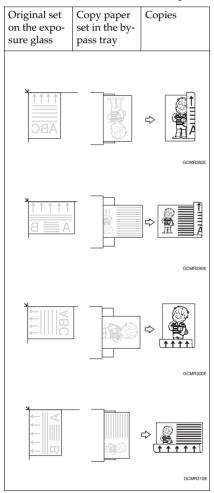
☐ If Duplex copying cannot be done because of paper problems, place paper on the bypass tray to copy on the front side, and once again copy on the backside.
