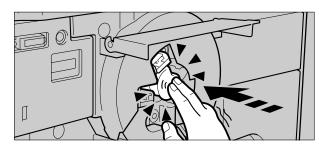
Pull out the toner cartridge while holding the hook.
