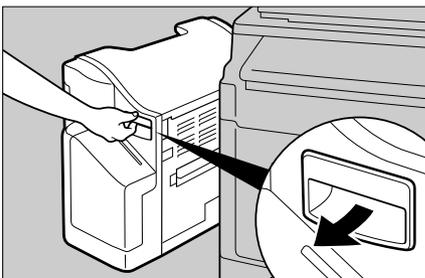
**6** Pull C4 to the left and rotate knob C1 clockwise to remove misfed paper.
