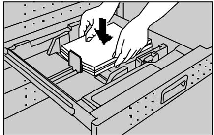
**4** While pressing the release lever on the front guide, slide the front and rear guides to paper size you want to use.
