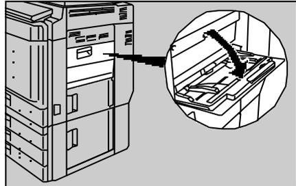
**5** Set the test pattern on the exposure glass (platen glass), and press the **Start** key.
