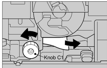
**4** If misfed paper is not fed, rotate knob C1 clockwise and remove misfeeds.
