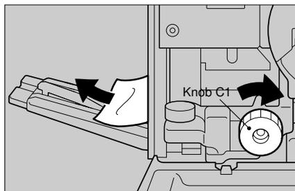
**5** If misfed paper is not fed by rotating knob C1, hold grip C3 while pressing lever C2 to pull out the fusing unit.
