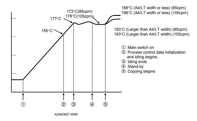
The CPU turns on all three fusing lamps after the main switch is turned on, with a one-second interval between each. This prevents the power from the AC line from dropping too quickly.
