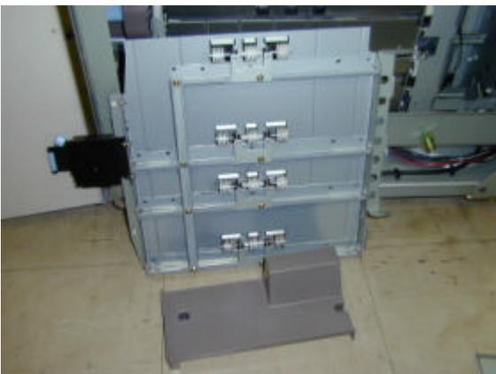
31. After installing the guide rail ass'y (A2943710) to the new inner cover (A2941524C), secure the inner cover to the mainframe (1 screw).
