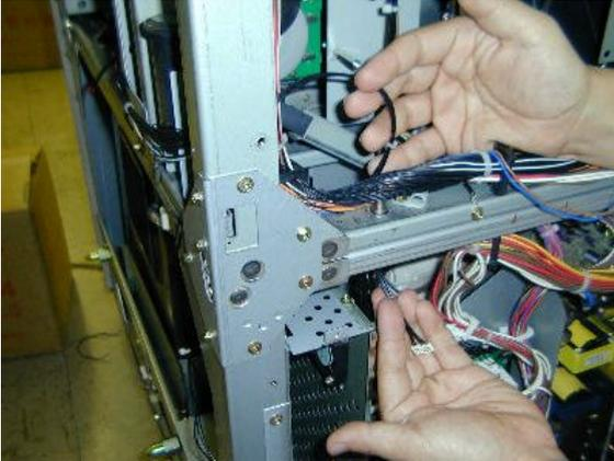
43. Connect the 6-pin connector end to the connector that sticks out of the screw hole on the upper right of the I/O board.
