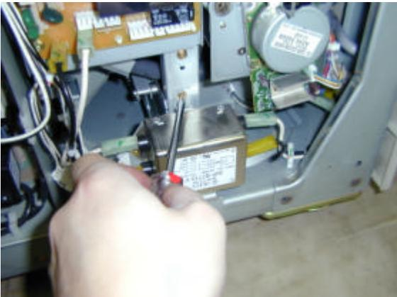
15. Remove the motor DC-5.1W. (1 connector, 2 screws)
