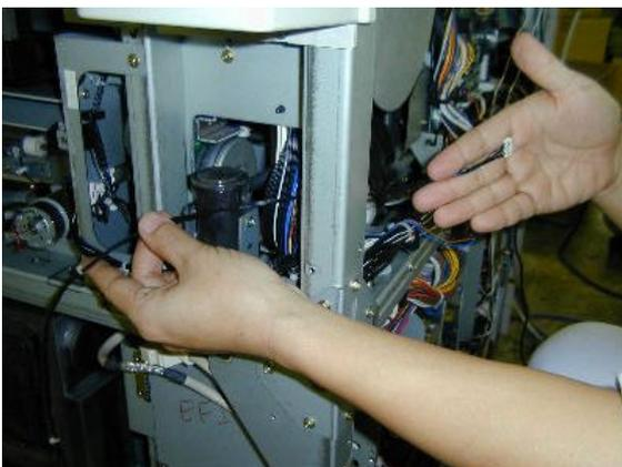
42. Pass the 6-pin connector end of the harness on the inside of the rear frame and lead it until it reaches the I/O board.
