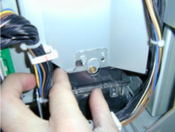
14. Pull the power plug out and remove the noise filter. (2 screws)
