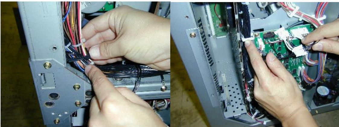
48. Fasten the relay connector side of the short pump harness using the clamp near the rear vertical frame support and the clamp underneath the I/O board.
