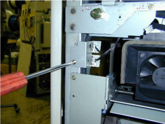
28. Install the toner suction pump to the pump bracket. (2 M4x8 tapping screws with washers)
