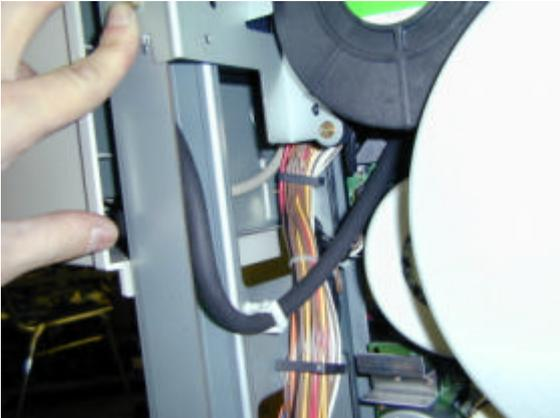
7. Remove the cap [A] of the tube joint case [B] at the end of the Ö12.4-silicon tube on the right side of the main frame.
