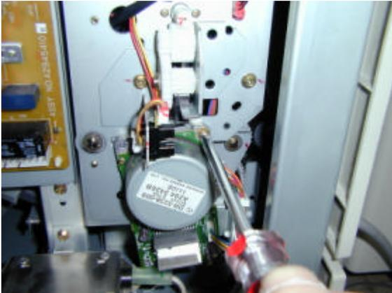
16. Remove the snap ring of the toner transport screw and slide the toner transport screw joint over to the left.
