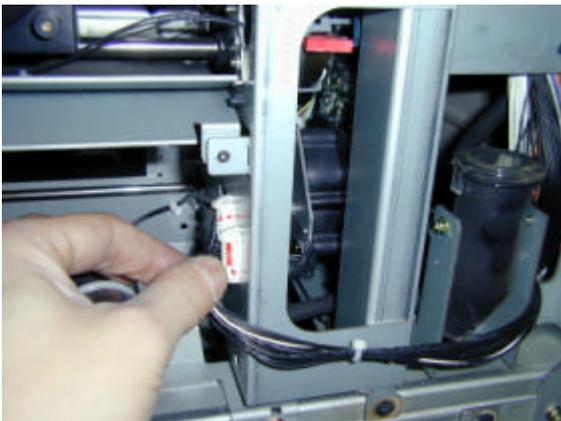
6. Remove the two-Ö6 tubes. Hook the upper end of the tube on the machine frame as shown to prevent toner dropping.
