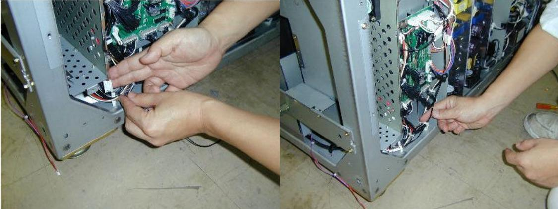
49. Connect the other end of the harness to the connector that sticks out of the upper right screw hole in the I/O board. This I/O board connector has 3 lines running to the I/O board and is marked red.
