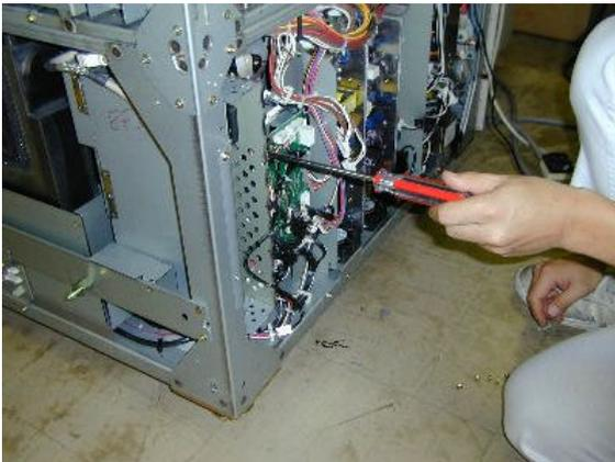
41. Orient the long harness so that the forked end is facing forward, and the end with the 6-pin, white connector is facing back. Pass the harness inside the vertical frame support (rear side, upper right).
