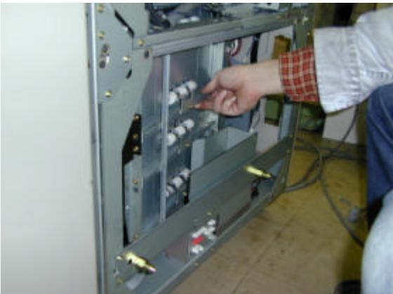
34. Set the toner collection bottle (A2943700) in the mainframe and attach the tube (12mm diameter).
