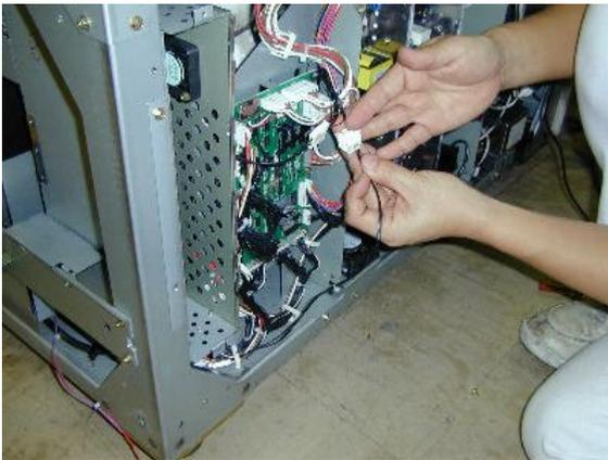
50. Connect the bottle set sensor connector to the short pump harness relay connector, located on the back face of the mainframe. To prevent the harness from getting pinched between moving parts or other components, remove the slack from the harness with the clamps if necessary.
