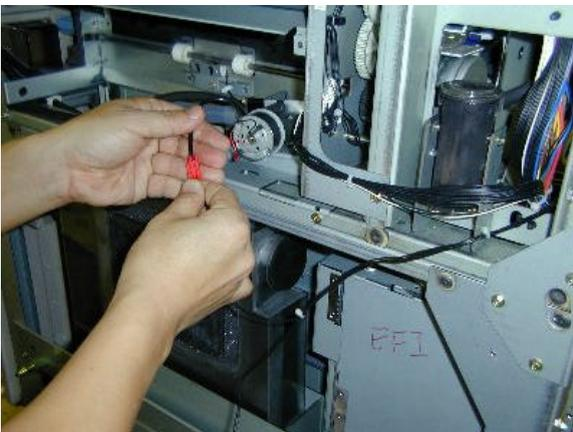
45. Connect the other end of the fork (white connector) to the connector on the pump unit drive sensor (photo interruptor type). Reinstall the pump bracket.
