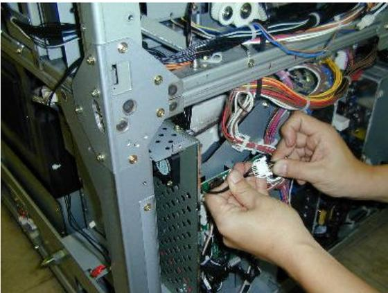
44. For the other end of the long pump harness (the forked end), remove the pump bracket (1 screw) and connect the red connector to the pump motor harness.
