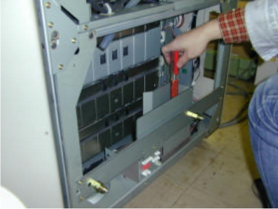
32. Attach the guide rail in the enhancement kit to the inner cover (A2941524B) in the mainframe, then install the two-part assembly in the mainframe (see photo below).
