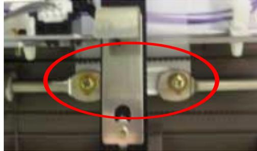
5. Rotate the R7 knob until the upper stay lightly contacts the adjustment board.
