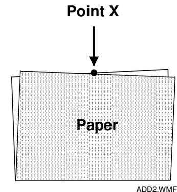
16. Repeat Steps 12 and 13 above, and if A, B, C or D is still above 2mm, go on to Step 17. If A, B, C, and D are all 2 mm or less, go on to step 19.
