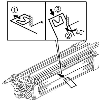
6. Rotate the development roller about 10 mm (about ½”) toward you, then vacuum away any paper dust or developer that falls away from the roller.
