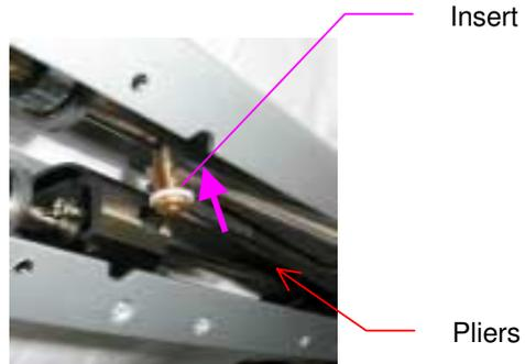
5. Secure the new punch head in place, holding it with a pair of needle-nosed pliers (1 screw).
