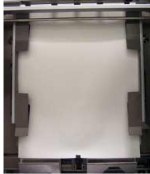
3. By manually moving the stack-feed out belt on the rear side of the unit, bring the adjustment board up until its edge is about at the top edge of the upper stay.
