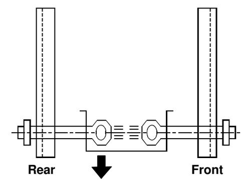
10. Bring the front jogger fence flush against the edge of the board, then adjust the front fence shaft until the board/fence gaps on both sides are:
