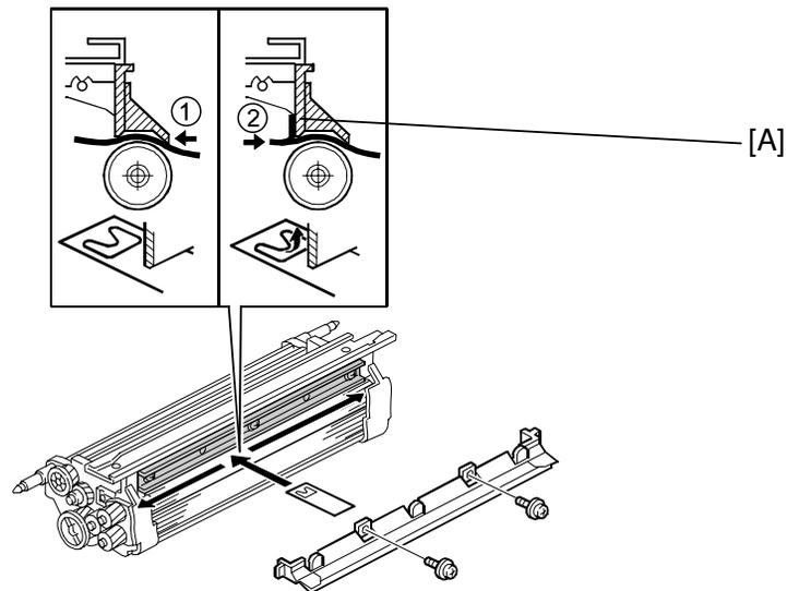
4. Slide the tool left and right several times, all the way the to the left and right ends of the gap.
