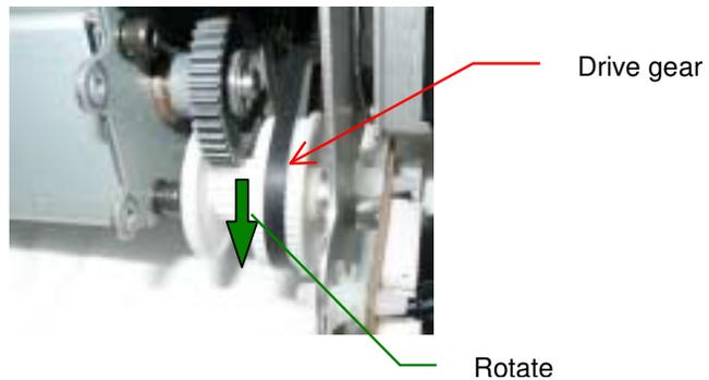
**NOTE:** Do not forcibly rotate the gear. If it is difficult to rotate, replace the entire punch unit.
