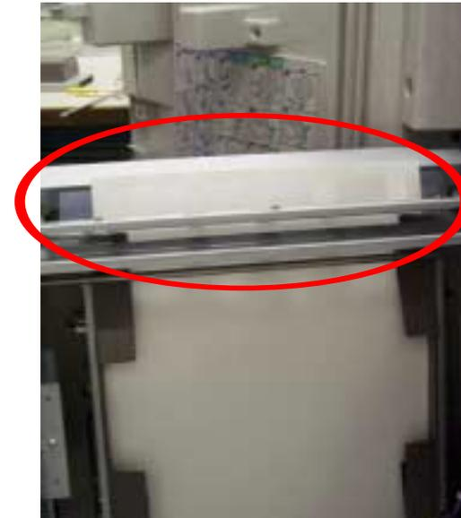
4. Loosen the 2 screws for the lower jogger shafts.
