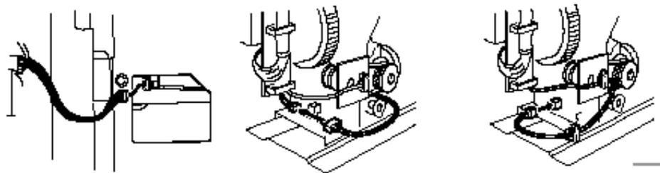
4. Remove the drive section from the toner bank unit (5 screws).
