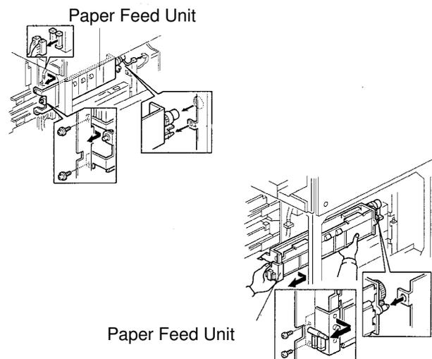
3. Remove the sensor bracket.
