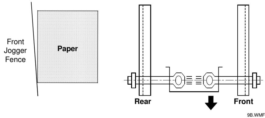
11. Tighten the screw for the front jogger fence all the way.
