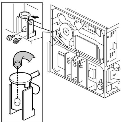
4. Remove any clogged toner through the upper hole of the tube joint using a vacuum cleaner.
